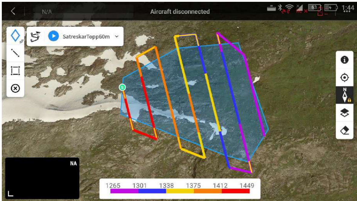
Figure 22. Flight route while LiDAR scanning desired polygon (blue). Flight lines are colored according to colorbar illustrating altitude above sea level (meters).
