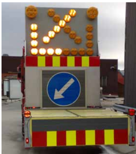
Figure 4.3 Warning panel on a motor vehicle with crash cushion.
