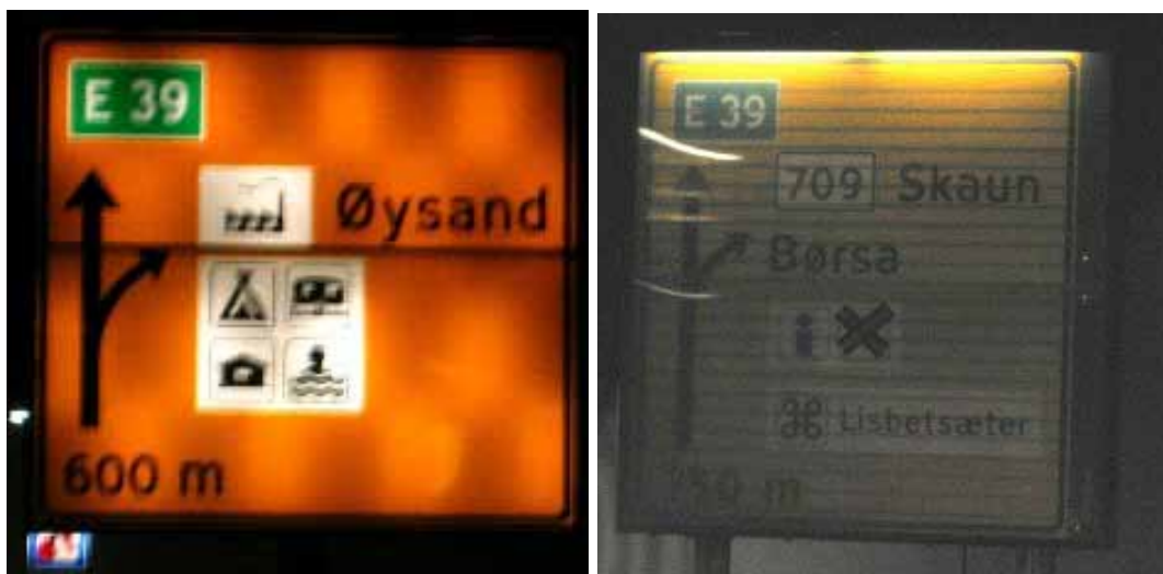
Figure 1.14 Examples of internally illuminated road traffic signs with bad luminance evenness.
