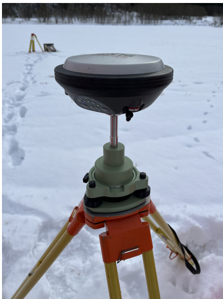
(a) The positioning measurement of tripods With RTK rover
