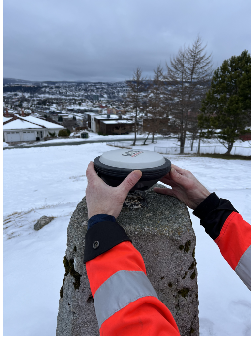
Figure 4.7: The known point Moholt measured for accuracy investigation of the RTK GNSS equipment
