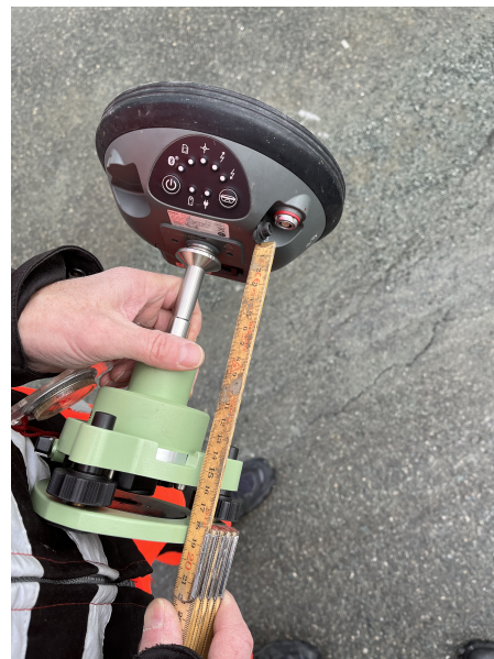
(b) Height measured from RTK to tripod
