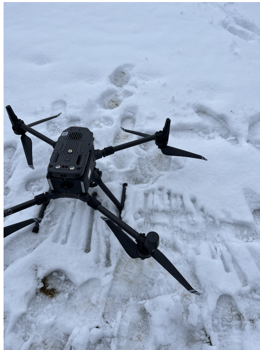
Figure 4.5: The UAV DJI Matrice 300 leaving marks in the snow showing indicating change of landing position between each session
