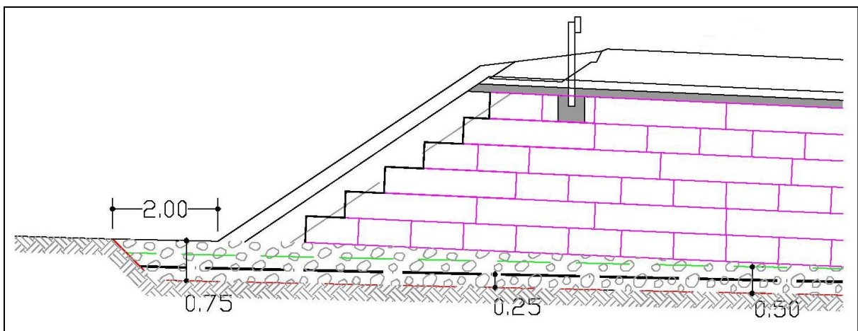
Figure 57: Material placement above subsoil in Athens-Thessaloniki highway
