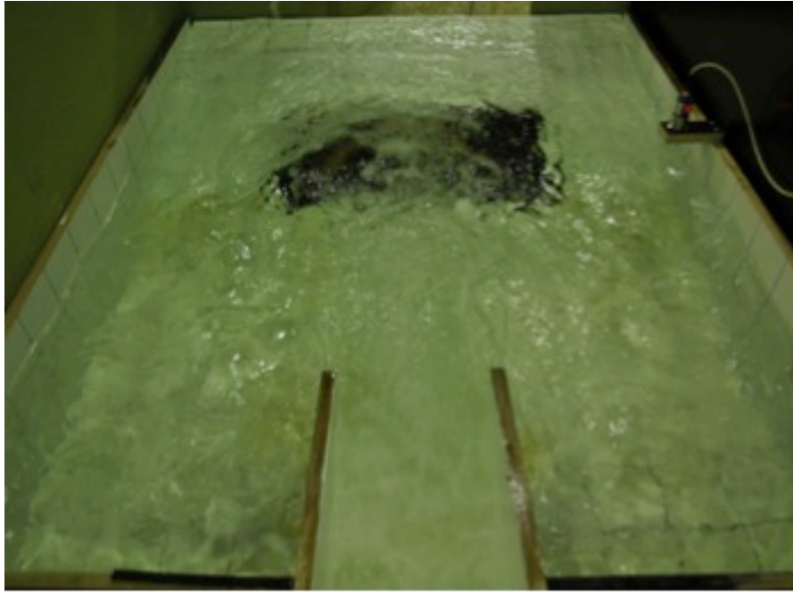
Figure 5.8 Overtopping basin edge for inlet with wingwalls and Q = 16 \text{ l/s}
