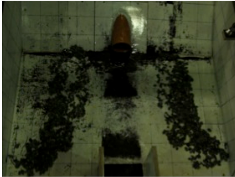
Figure 5.18 Symmetric deposition of sediments added all at once for a projecting inlet with Q = 12 l/s
