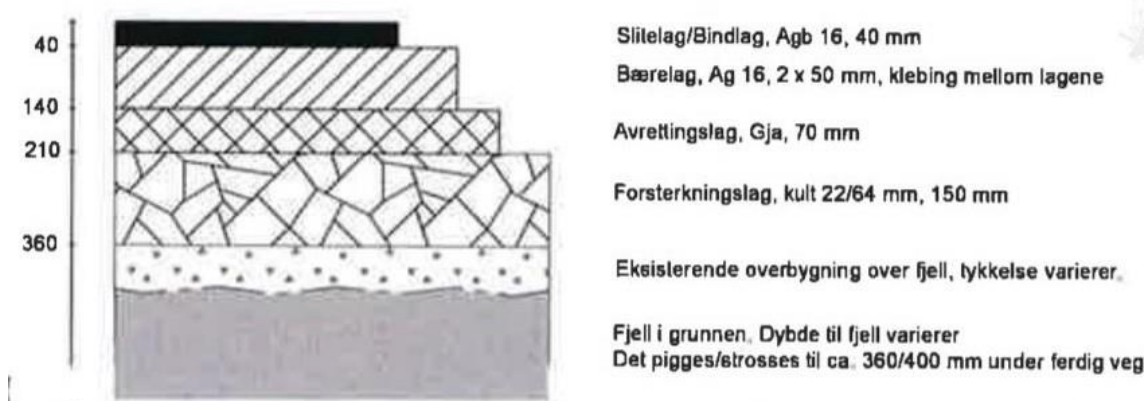
Figur 19, detalj overbygning tunnel
