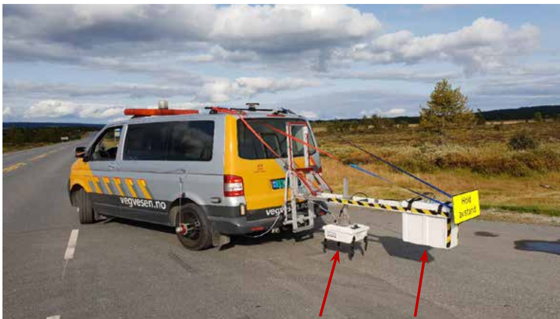
Figur A3.14 Georadarantenner. (Foto: Haris Brcic)
