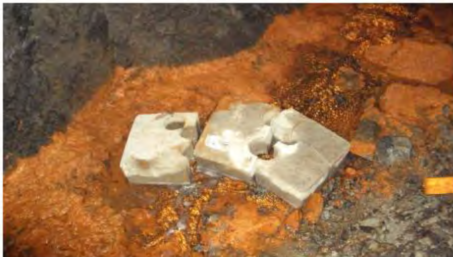
Figure 7: Ditch A with samples cast in plastic moulds. Later on the water level became higher. Cores were first extracted for reference.
