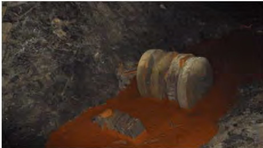
Figure 5: Ditch A showing panels and smaller plate-shaped samples exposed to running water with extensive iron bacterial accumulation. Placed upright in order to investigate possible different effects of water and damp tunnel air.
