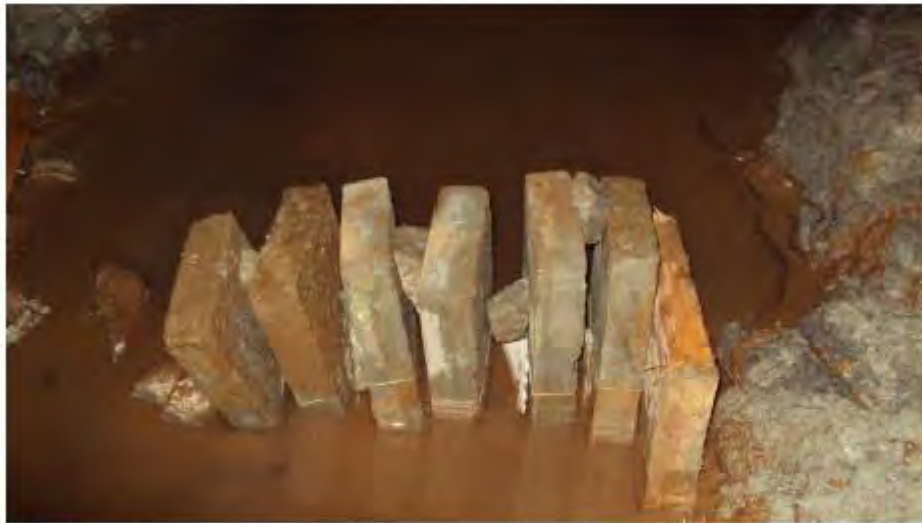
Figure 6: Ditch B showing plate-shaped samples exposed to iron and manganese enriched stagnant water.
