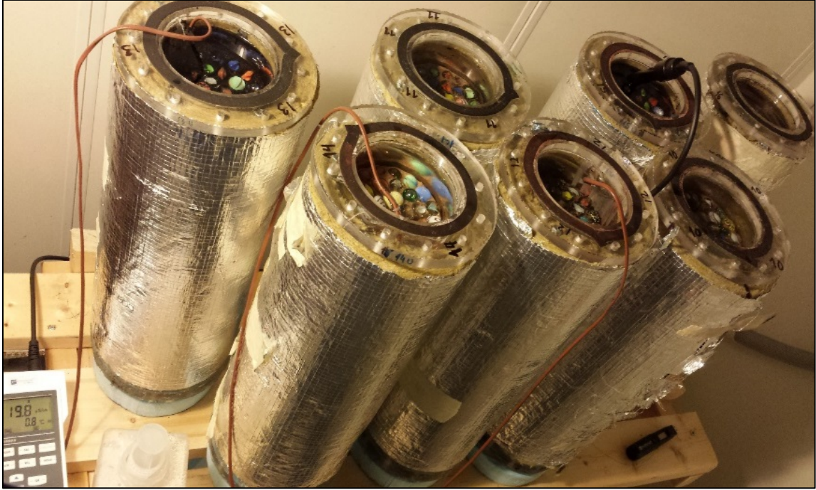
Figure 4. Columns in the cold chamber under freezing/thawing simulation
