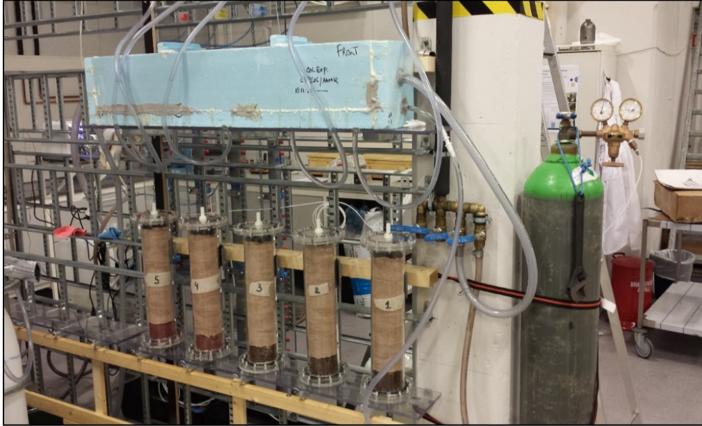
Figure 3 Setup for measurement of K-sat at room temperature
