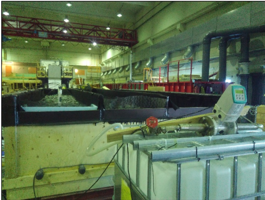
Figure 9. Inlet tank with needle valve and flowmeter.
