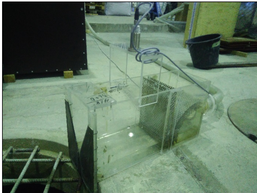
Figure 11: The V-notch weir with microsensor.
