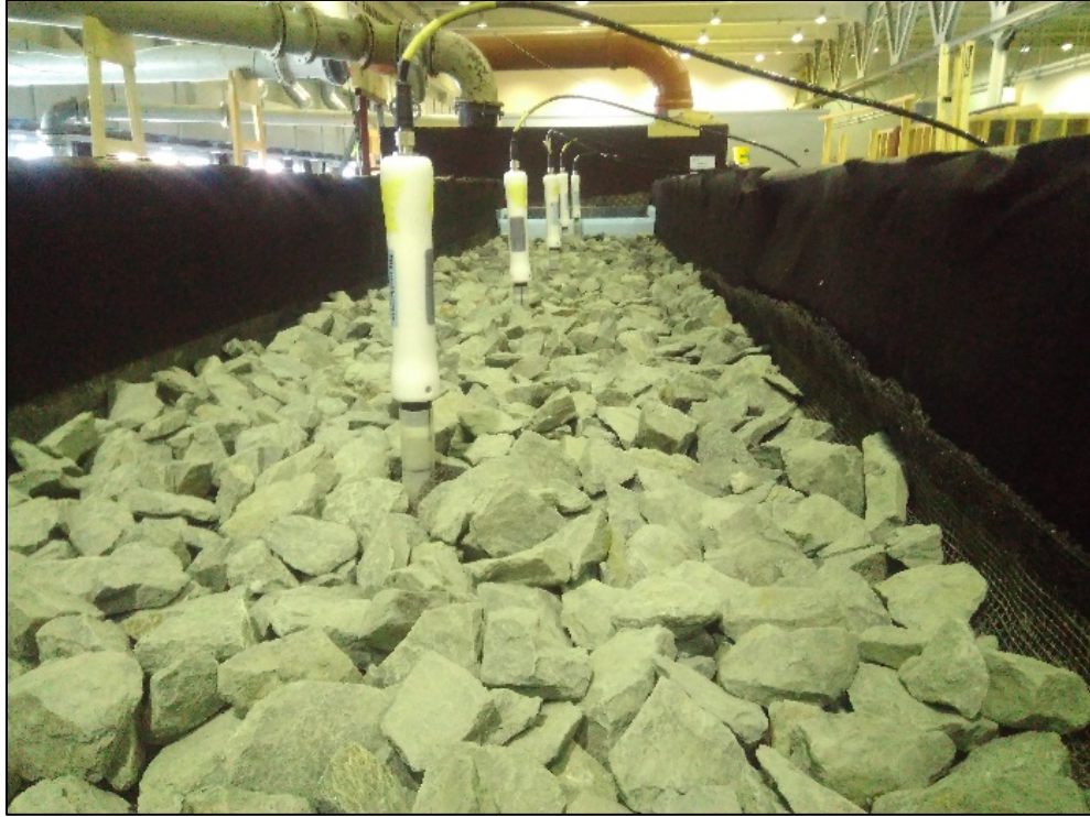
Figure 12. Soil moisture probes along the filter protected with boulders.
