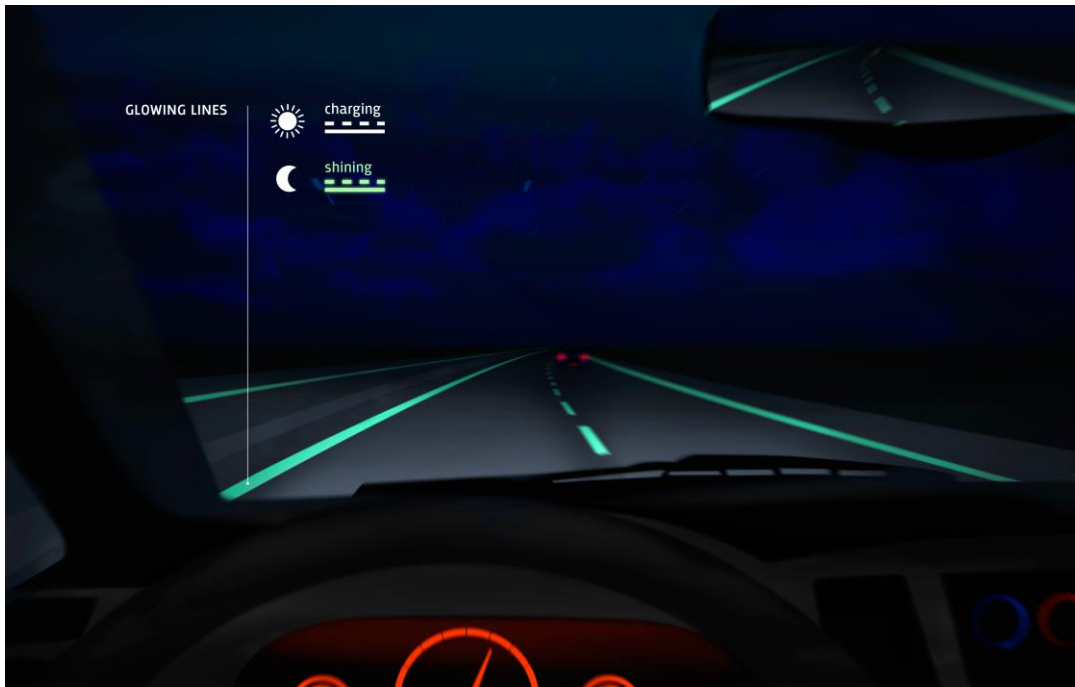
Figure 18. Glowing road markings for smart roads. (Image from www.smarthighway.net )
