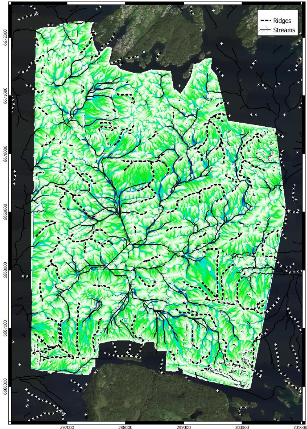
> Figure 5-28 Flow accumulation from watershed calculation of bedrock, overlain with ridges and streams calculated by NGI, ref. [10].
