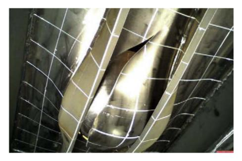
> Figure 3-2 Experimental test. Indentation of panel with 2 HP-stiffeners [17].
