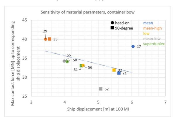
Figure 7-4 Sensitivity of material parameters, impact container bow-pontoon
