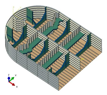
> Figure 4-6 Corrugated pontoon finite element model
