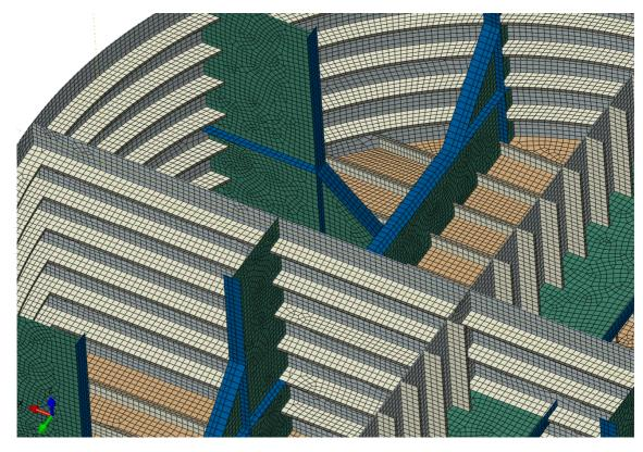
> Figure 4-17 Detailed mesh of the pontoon
