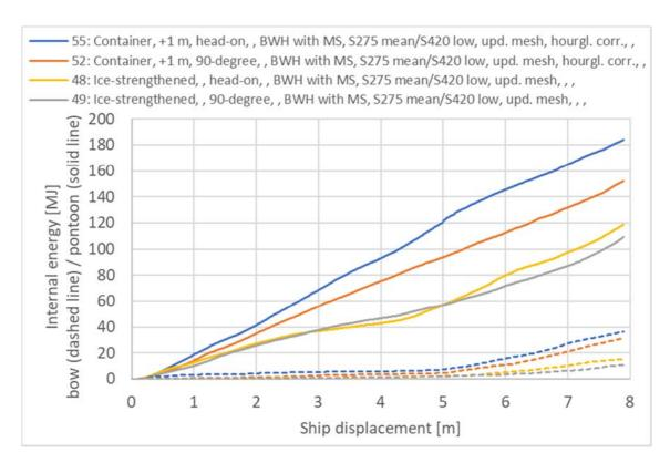
> Figure 5-12 Internal energy [MJ] impact bow-pontoon
