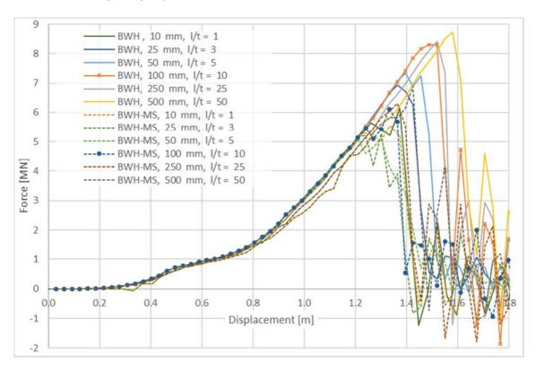
> Figure 3-7 Sensitivity study for BWH. MS – mesh scaling.
