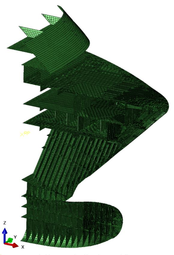
> Figure 4-13 Mesh of the ice-strengthened bow, shown cut in half
