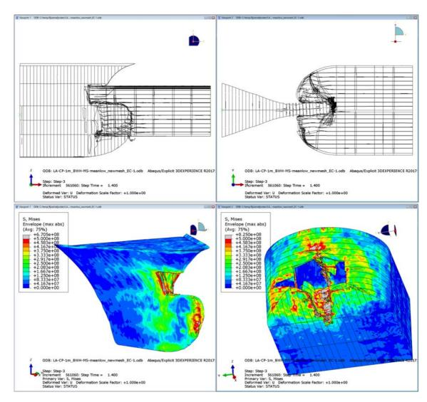
Figure 5-6 von Mises stress [MPa] load case A: Container bow at design draught (8.6 m), head-on impact on pontoon
