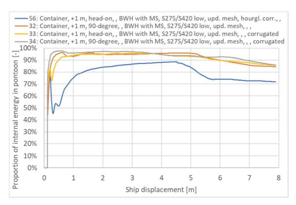
> Figure 5-30 Proportion of internal energy in pontoon [-] impact bow-pontoon, corrugated bulkheads
