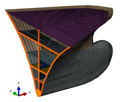
Figure 4-20 Boundary condition at the cut-off boundary of the ship bow
