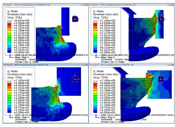
> Figure 5-34 von Mises stress [MPa] forecastle-column collision side view: 90-degree (upper), head-on (lower), container bow (left), ice-strengthened bow (right)
