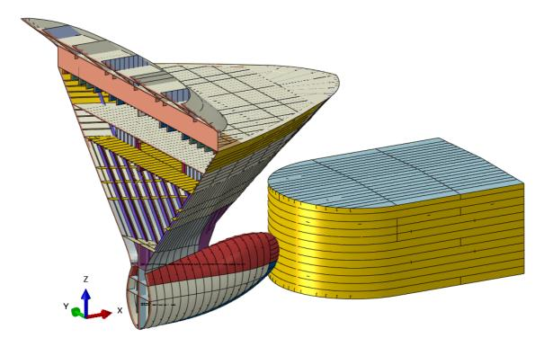
> Figure 4-5 Pontoon finite element model with ice-strengthened bow head-on impact
