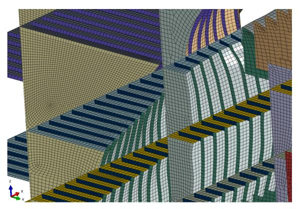
> Figure 4-15 Detailed mesh of the container bow
