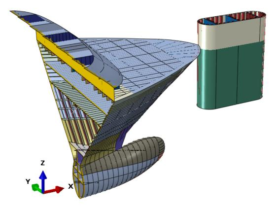
Figure 4-10 Column finite element model with ice-strengthened bow head-on impact
