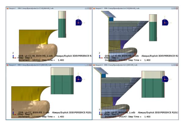
> Figure 5-5 Load cases A-D of forecastle-column collision side view: 90-degree (upper), head-on (lower), container bow (right), ice-strengthened bow (right)
