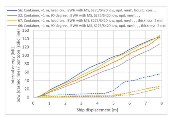
> Figure 5-22 Internal energy [MJ] impact bow-pontoon, plate thickness reduction
