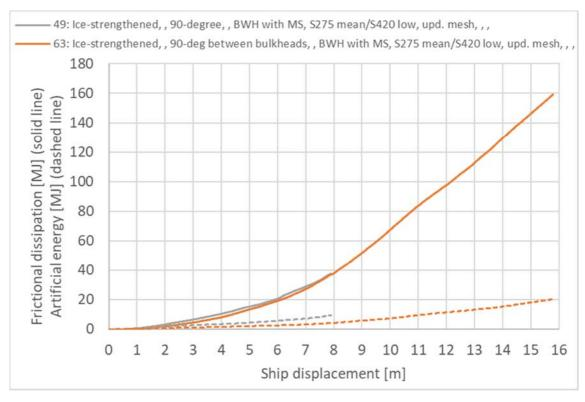
> Figure 5-17 Frictional dissipation and artificial energy [MJ] impact ice-strengthened bow-pontoon 90-degree on bulkhead or between bulkheads/frames
