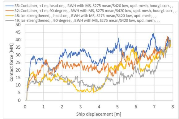
> Figure 5-11 Contact force [MN] impact bow-pontoon
