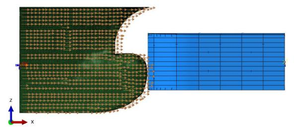
> Figure 4-22 Velocity applied to the container bow in step one
