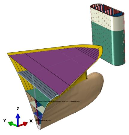
> Figure 4-9 Column finite element model with container bow 90-degree impact
