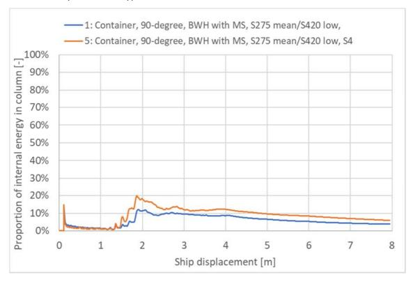
> Figure 5-44 Proportion of internal energy in column [-] impact forecastle-column, sensitivity of element type
