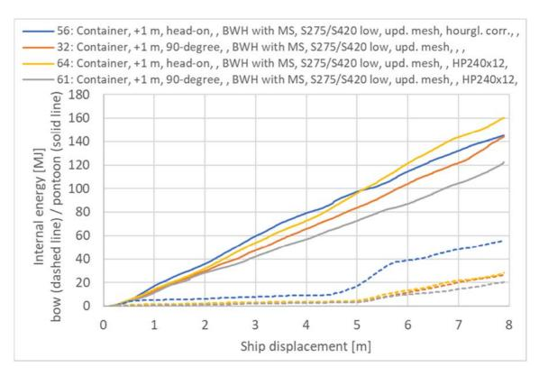
> Figure 5-23 Internal energy [MJ] impact bow-pontoon, stiffener reduction
