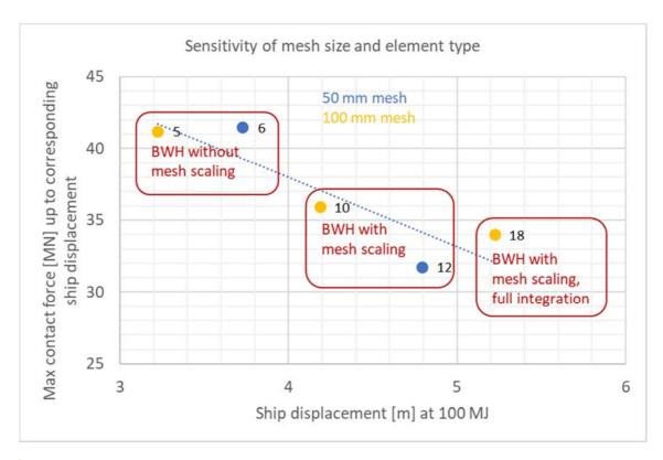
> Figure 7-7 Sensitivity of mesh size and element type
