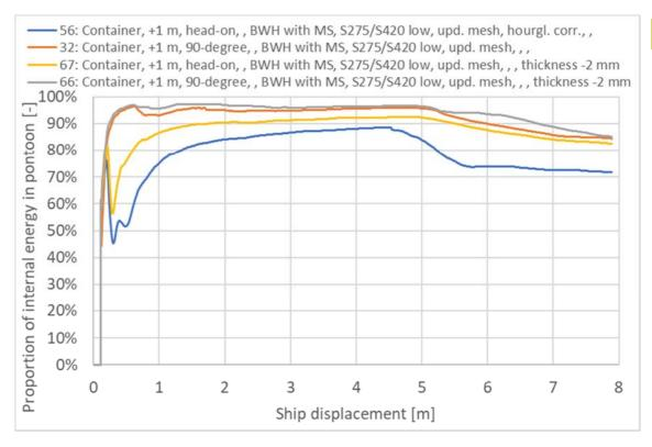
> Figure 5-28 Proportion of internal energy in pontoon [-] impact bow-pontoon, plate thickness reduction
