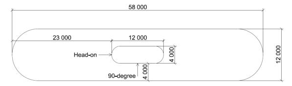
> Figure 5-32 Plan of smallest pontoon and column [mm]
