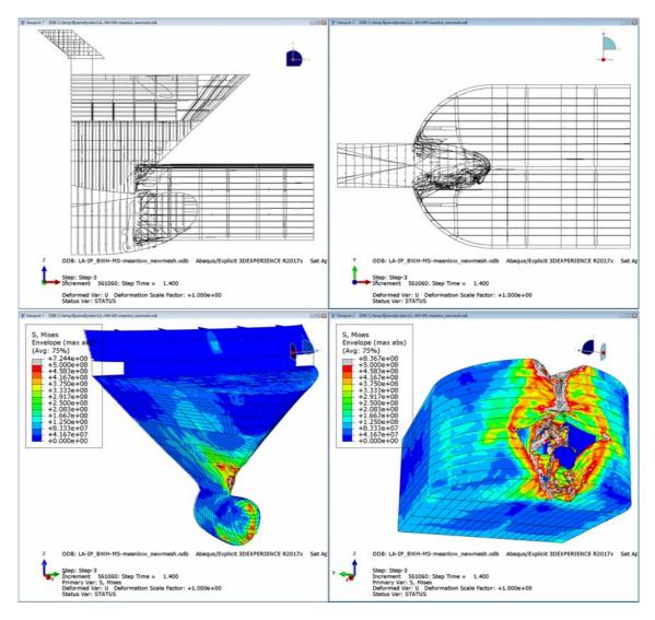
> Figure 5-8 von Mises stress [MPa] load case C: Ice-strengthened bow at design draught (6.8 m), head-on impact on pontoon
