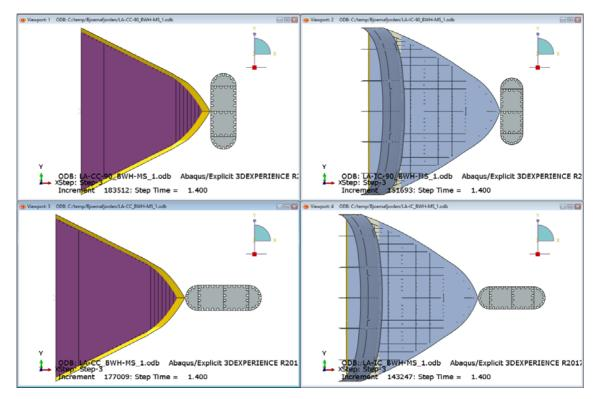
> Figure 5-4 Load cases A-D of forecastle-column collision seen from above: 90-degree (upper), head-on (lower), container bow (right), ice-strengthened bow (right)
