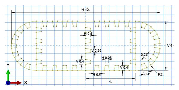
> Figure 4-8 Plan of the column, dimensions in [m]
