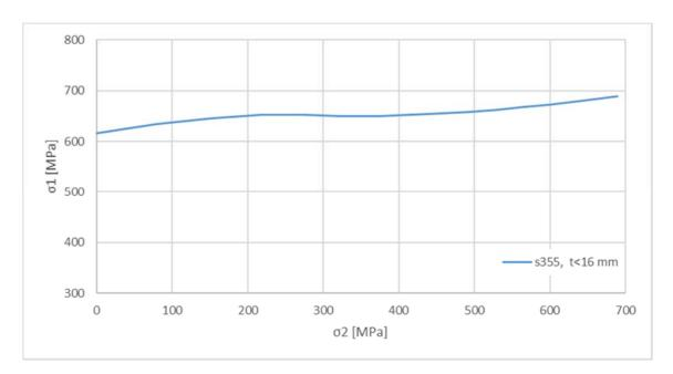
Figure 3-1 BWH failure criterion for plane-stress conditions. Exemplified with S355 steel.
