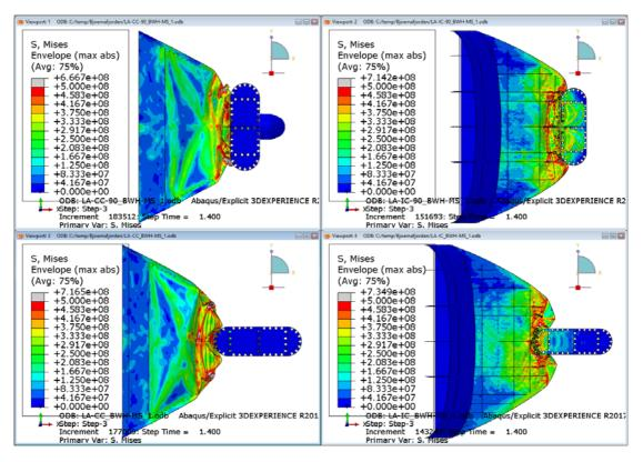
> Figure 5-33 von Mises stress [MPa] forecastle-column collision seen from above: 90-degree (upper), head-on (lower), container bow (left), ice-strengthened bow (right)
