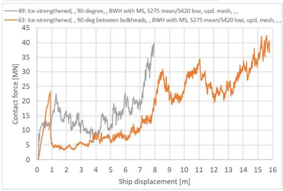
> Figure 5-15 Contact force [MN] impact ice-strengthened bow-pontoon 90-degree on bulkhead or between bulkheads/frames
