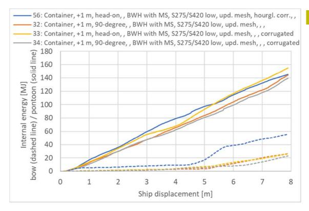
> Figure 5-24 Internal energy [MJ] impact bow-pontoon, corrugated bulkheads
