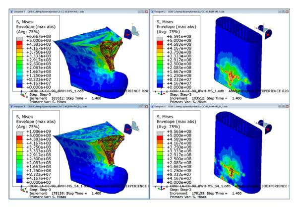
> Figure 5-40 von Mises stress [MPa] forecastle-column collision: Comparison reduced integration (upper) with full integration (lower), container bow (left), column (right)
