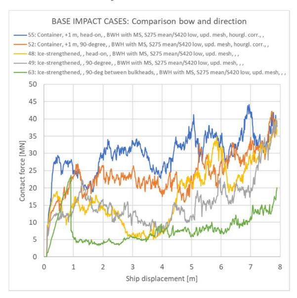
> Figure 7-1 Contact force [MN] impact bow-pontoon
