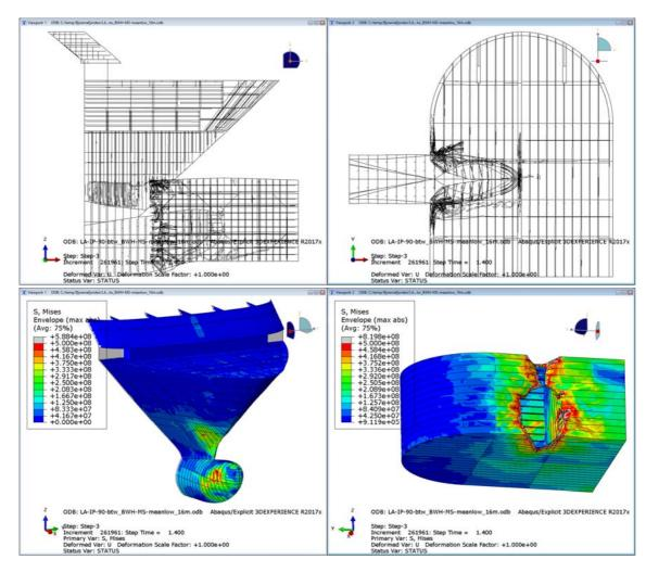
> Figure 5-10 von Mises stress [MPa] load case E: Ice-strengthened bow at design draught (6.8 m), 90-degree impact on pontoon between bulkheads and frames
