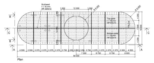
> Figure 4-1 Plan of the pontoon in axis 3, from drawing K7-057 [18]. The pontoon width has become slightly larger (17 m) than the pontoon geometry utilized in this report (16 m), but this is considered to have negligible influence on the results.
