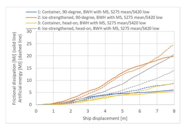
> Figure 5-37 Frictional dissipation and artificial energy [MJ] impact forecastle-column
