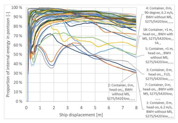
> Figure 7-9 Proportion of internal energy in pontoon [-] impact bow-pontoon, series name of the non-conservative simulations with low proportion of dissipated energy in the pontoon is displayed
