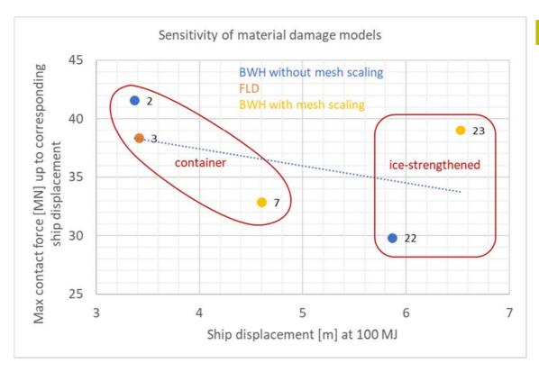
> Figure 7-6 Sensitivity of material damage models
