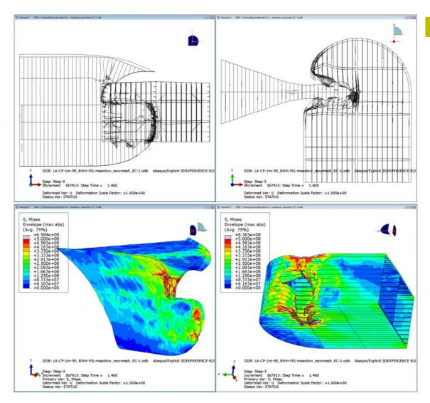
> Figure 5-7 von Mises stress [MPa] load case B: Container bow at design draught (8.6 m), 90-degree impact on pontoon
