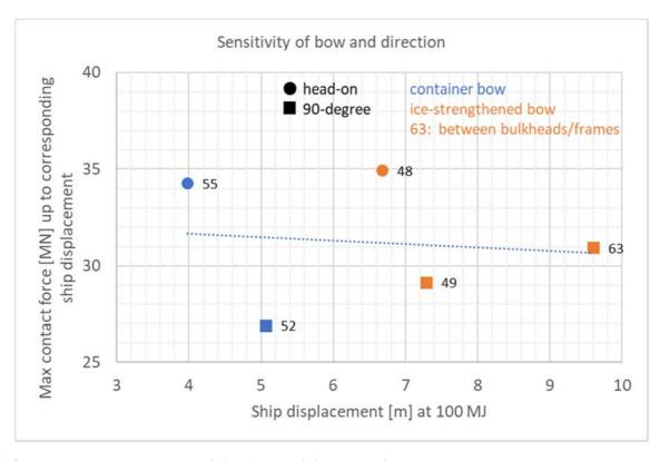
> Figure 7-2 Sensitivity of ship bow and direction of impact
