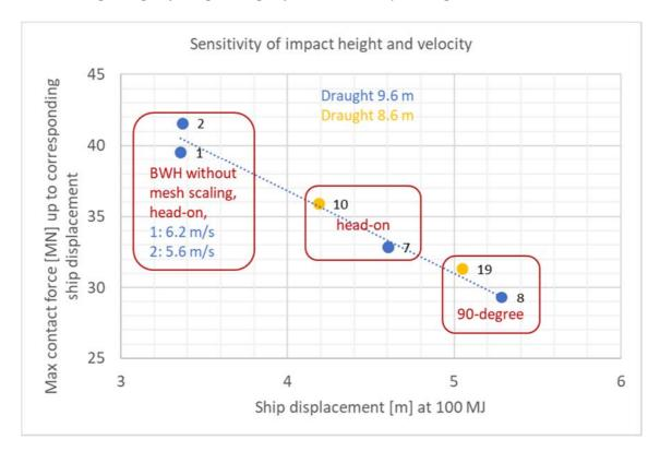
> Figure 7-8 Sensitivity of impact height and velocity, impact container bow-pontoon
