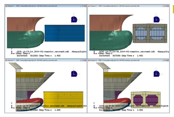
> Figure 5-3 Load cases A-D of bow-pontoon collision side view: Container bow (upper), ice-strengthened bow (lower), head-on (left), 90-degree (right)
