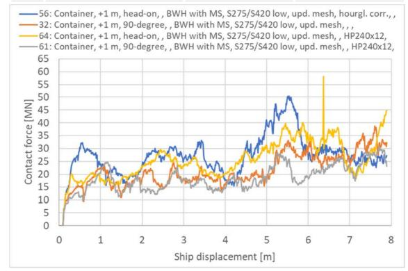
> Figure 5-20 Contact force [MN] impact bow-pontoon, stiffener reduction
