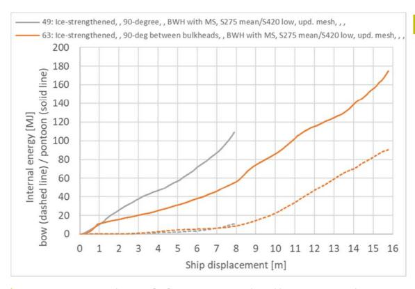
> Figure 5-16 Internal energy [MJ] impact ice-strengthened bow-pontoon 90-degree on bulkhead or between bulkheads/frames
