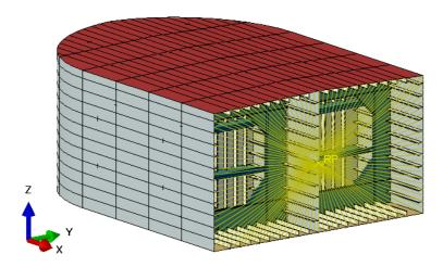
> Figure 4-19 Boundary condition at the cut-off boundary of the pontoon
