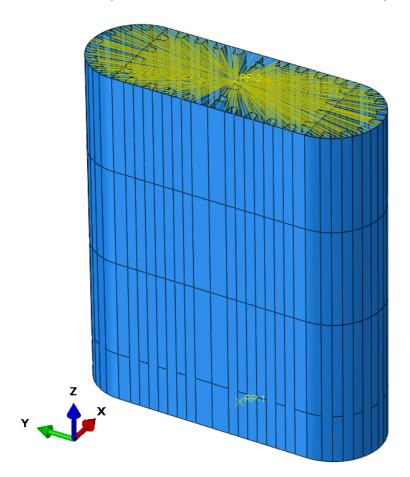
> Figure 4-21 Boundary conditions at the cut-off boundaries of the column
