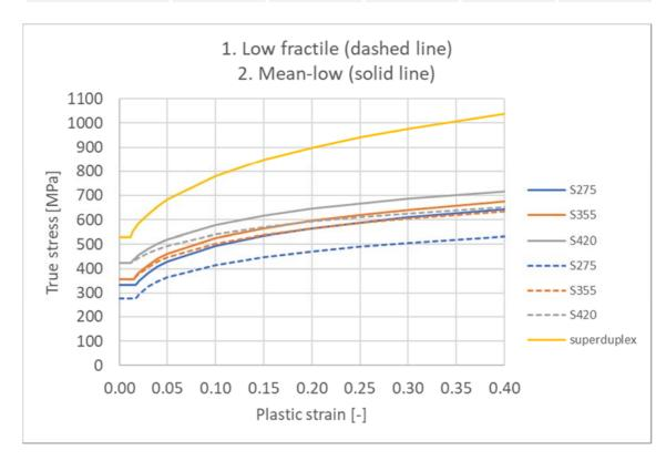
> Figure 4-11 True stress-strain curves of the steel materials, solid lines define the base case materials utilized
