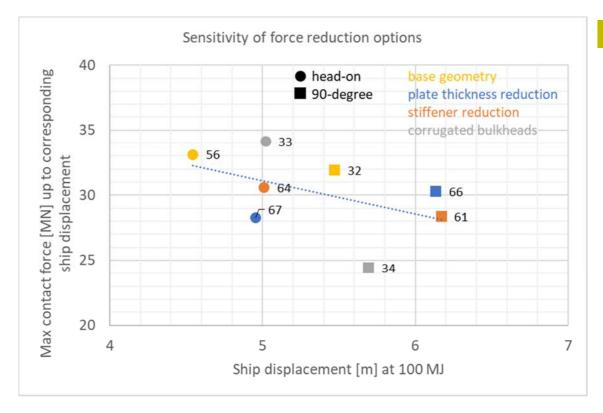
> Figure 5-31 Sensitivity of force reduction options, impact container bow-pontoon
