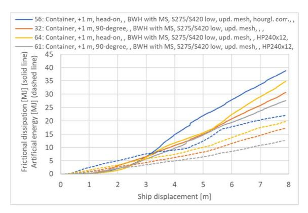
> Figure 5-26 Frictional dissipation and artificial energy [MJ] impact bow-pontoon, stiffener reduction
