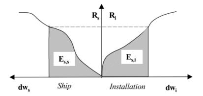
> Figure 2-1 Force equilibrium based on force-displacement curves (from [5])
