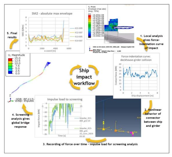
> Figure 2-2 Ship impact workflow. Local analysis: step 1. Global analysis and post-processing step 2-5.
