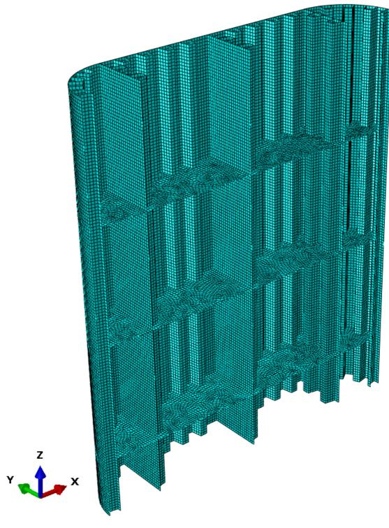
> Figure 4-18 Mesh of the column, shown cut in half
