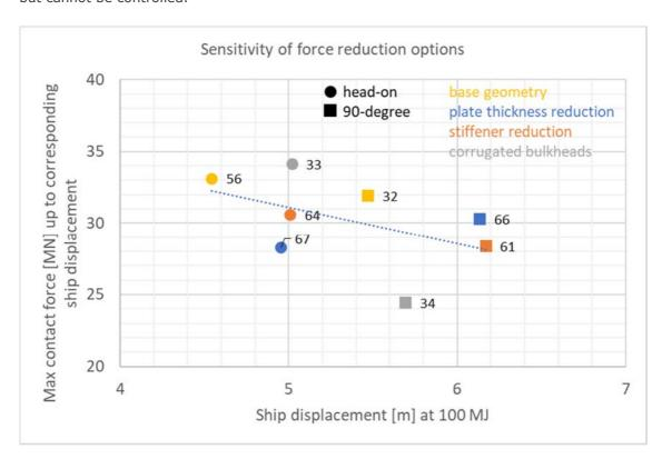
> Figure 7-3 Sensitivity of force reduction options, impact container bow-pontoon
