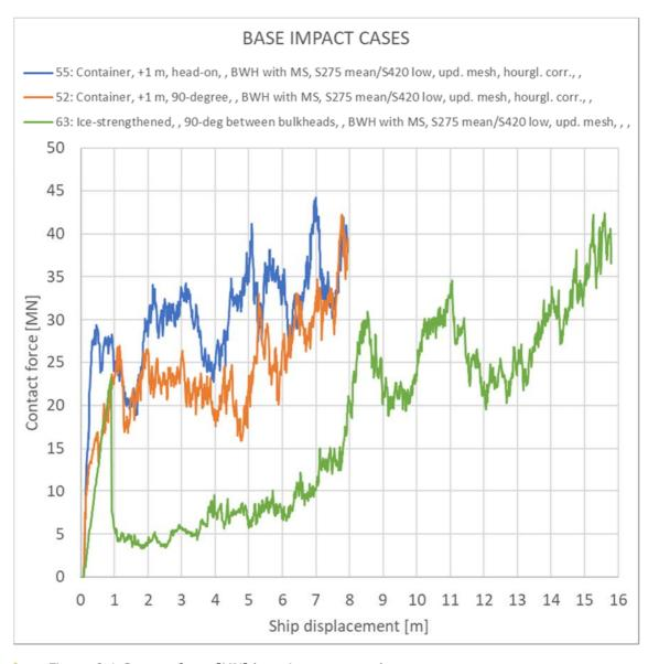
> Figure 6-1 Contact force [MN] base impact cases bow-pontoon
