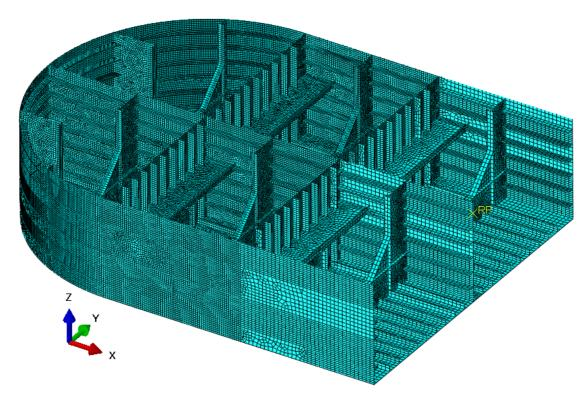
> Figure 4-14 Mesh of the pontoon, shown cut in half
