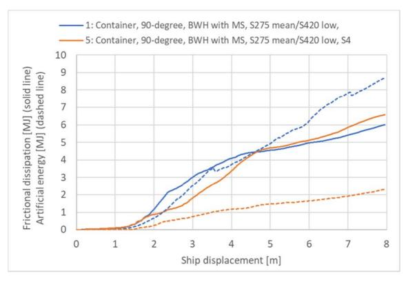
> Figure 5-43 Frictional dissipation and artificial energy [MJ] impact forecastle-column, sensitivity of element type
