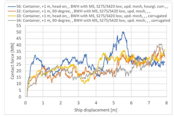
> Figure 5-21 Contact force [MN] impact bow-pontoon, corrugated bulkheads
