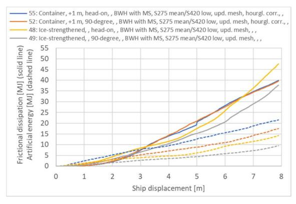
> Figure 5-13 Frictional dissipation and artificial energy [MJ] impact bow-pontoon
