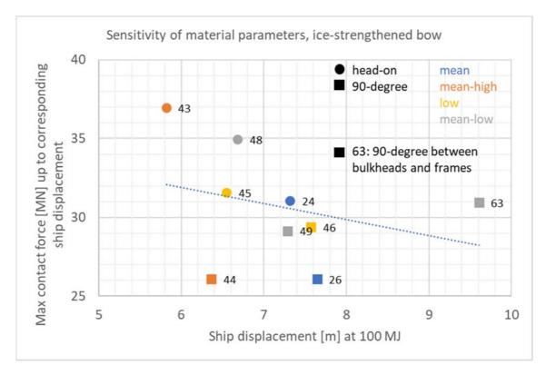
Figure 7-5 Sensitivity of material parameters, impact ice-strengthened bow-pontoon
