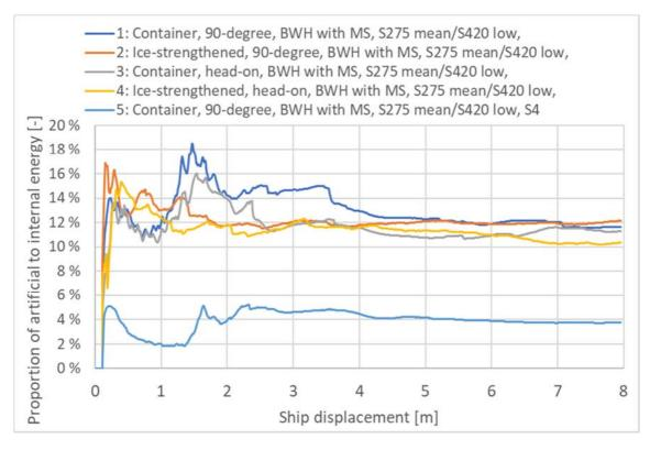
> Figure 5-39 Proportion of artificial energy to internal energy [-] impact forecastle-column: The low curve is with full integration
