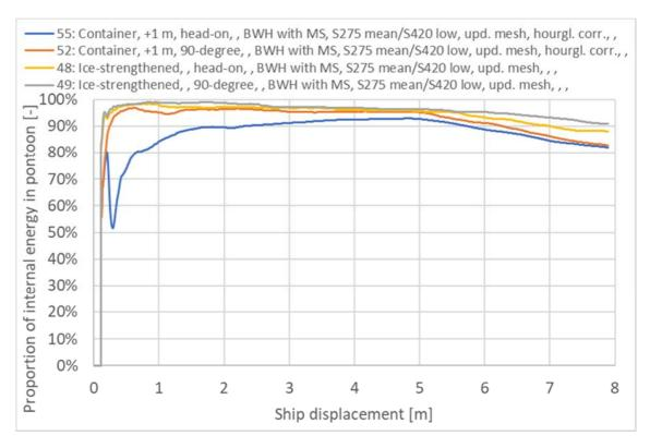
> Figure 5-14 Proportion of internal energy in pontoon [-] impact bow-pontoon
