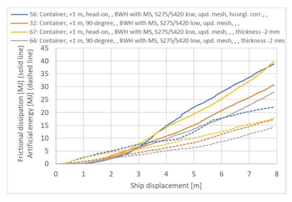
> Figure 5-25 Frictional dissipation and artificial energy [MJ] impact bow-pontoon, plate thickness reduction
