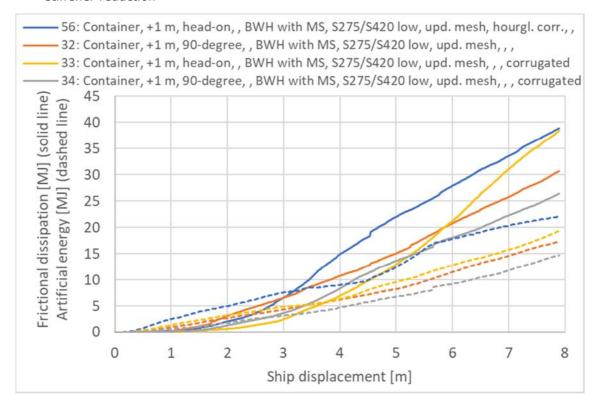
Figure 5-27 Frictional dissipation and artificial energy [MJ] impact bow-pontoon, corrugated bulkheads
