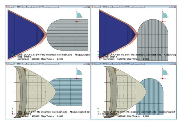
> Figure 5-2 Load cases A-D of bow-pontoon collision seen from above: Container bow (upper), ice-strengthened bow (lower), head-on (left), 90-degree (right)
