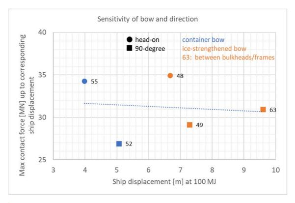
Figure 2 Sensitivity of ship bow and direction of impact
