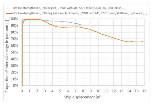
Figure 5-18 Proportion of internal energy in pontoon [-] impact ice-strengthened bow-pontoon 90-degree on bulkhead or between bulkheads/frames
