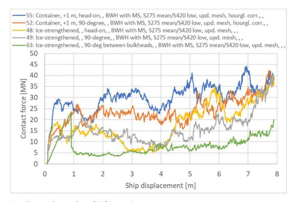
> Figure 1 Contact force [MN] impact bow-pontoon
