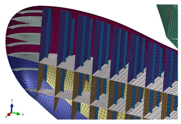
> Figure 4-16 Detailed mesh of the ice-strengthened bow
