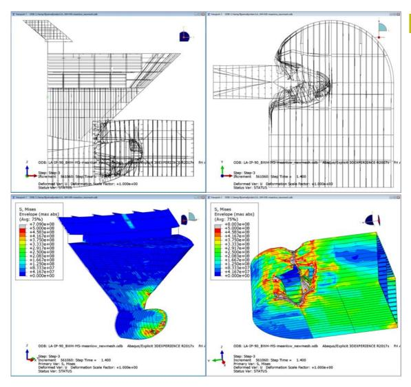
> Figure 5-9 von Mises stress [MPa] load case D: Ice-strengthened bow at design draught (6.8 m), 90-degree impact on pontoon
