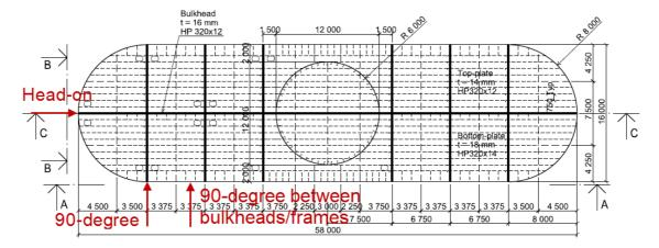
Figure 5-1 Illustration of head-on and 90-degree directions
