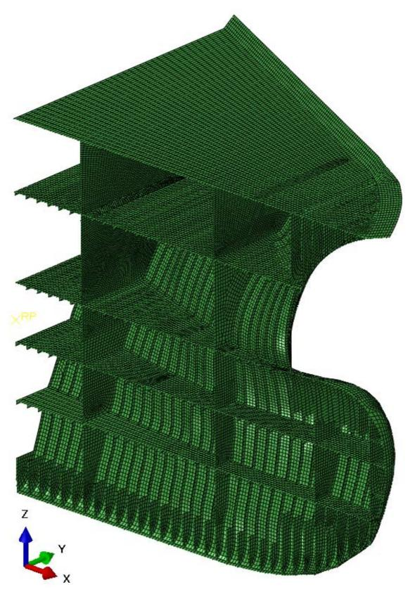
> Figure 4-12 Mesh of the container bow, shown cut in half
