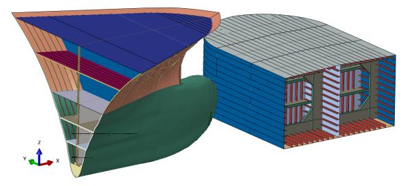
Figure 4-4 Pontoon finite element model with container bow 90-degree impact
