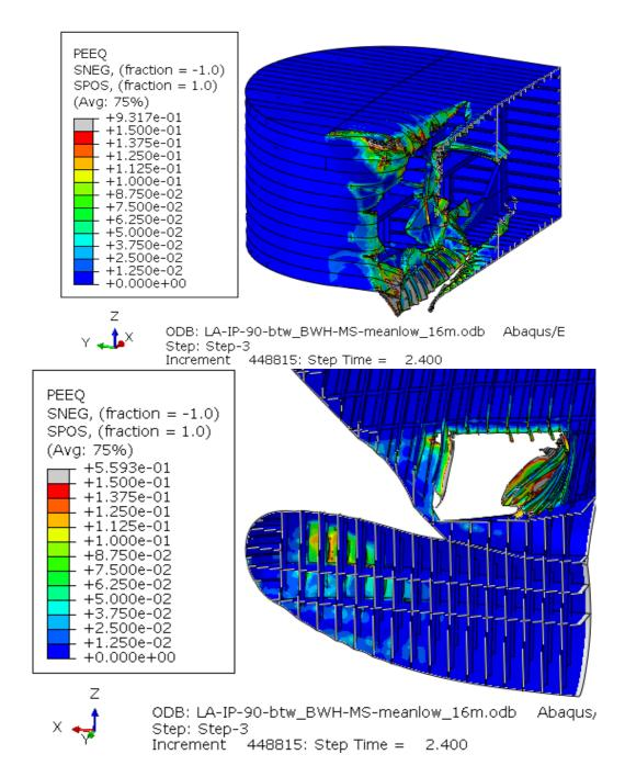
Figure 6-4 Damaged ship and pontoon at 13 m indentation between ship and pontoon.
