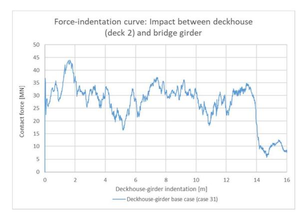
> Figure 3-5 Force-indentation curve for deckhouse-girder impact. Obtained from local analysis and used for all girder impacts in this report.
