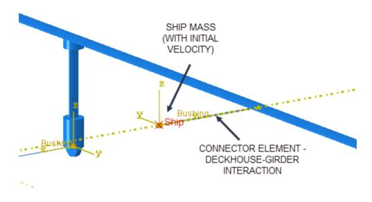
Figure 4-7 Ship impact setup for impact on bridge girder. Note that the length of the connector is only for visual representation. Above with beam profile rendering, below without.
