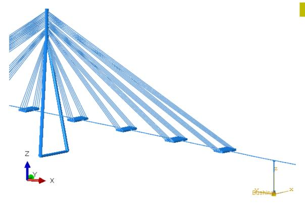
> Figure 4-2 Global FE-model showing area around the navigation channel. Beam profiles for tower, girder and pontoon columns are rendered.
