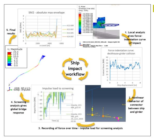
Figure 2-3 Ship impact workflow. Step 1: Local analyses as in report [3] and [4].
