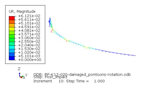
Figure 6-6 Post impact static state, pontoons in axis 3, 12 and 20 (will not happen at the same time). Scale factor 15 in plot.
