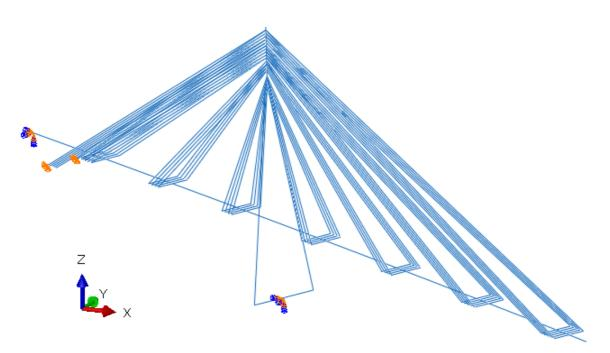
Figure 4-3 Boundary conditions on cable stayed bridge, global FE-model. The bridge girder is fixed towards the southern abutment, and first cable group from south abutment is pinned to the ground. The tower is fixed to "the ground".
