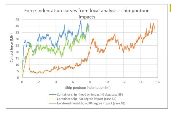
Figure 3-4 Force-indentation curve for ship-pontoon impacts. Head-on impacts for container ship and 90-degree impact from both container ship and ice-strengthened bow. Obtained from local analysis and used for all pontoon impacts in this report.
