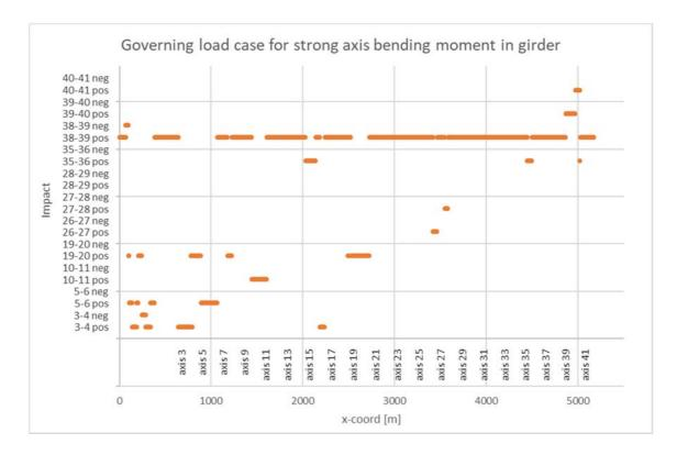
Figure 5-4 Governing impacts along girder for strong axis bending moment in girder, based on screening impulse analysis.
