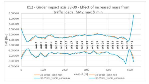
Figure 6-8 Effect of traffic loads on bridge. Comparison between two girder impacts between axis 38 and 39 with different girder densities. Max and min strong axis bending moment in girder, SM2 [Nm].
