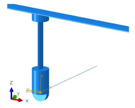
Figure 4-4 General pontoon represented with a connector "fixed to ground" with vertical and rotational stiffness. The remaining degrees of freedom are free to move/rotate. Structural mass and added mass are applied as point masses/inertias in the same point as the connector.
