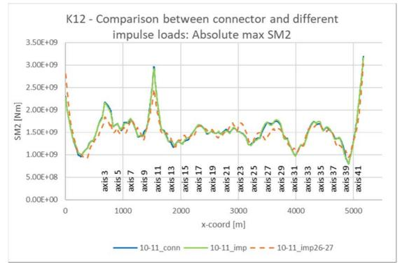
Figure 5-7 Comparison between screening result from connector analysis g10-11, impulse analysis based on connector analysis g10-11 and impulse load based on connector analysis from similar impact g26-27 – absolute max strong axis bending moment in girder, SM2 [Nm].
