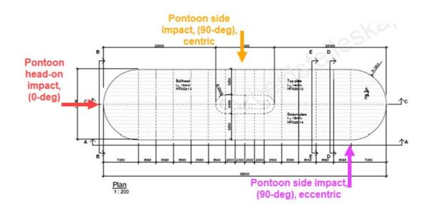
*Figure 3-3 Illustration of the three pontoon impacts considered in this study.*
