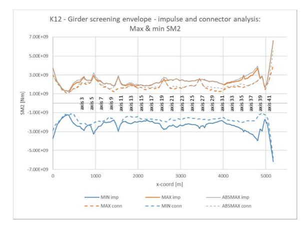
Figure 5-5 Comparison between screening results from impulse analysis (solid lines) and from connector analysis (dashed lines) – strong axis bending moment in girder, SM2 [Nm].
