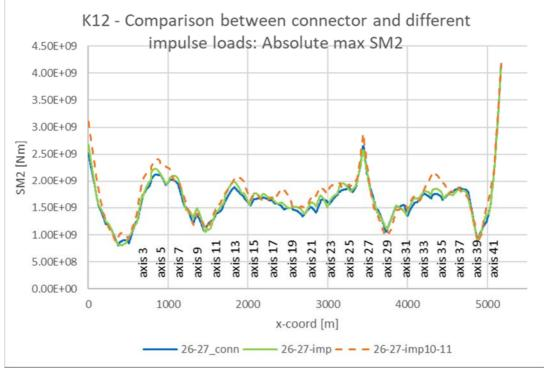
Figure 5-8 Comparison between screening result from connector analysis g26-27, impulse analysis based on connector analysis g26-27 and impulse load based on connector analysis from similar impact g10-11 – absolute max strong axis bending moment in girder, SM2 [Nm].
