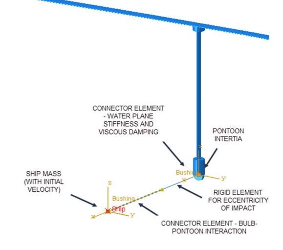
Figure 4-6 Ship impact setup for a head-on (0-deg) ship impact on pontoon in axis 3 (for an older model version). Note that the length of the connector is only for visual representation.
