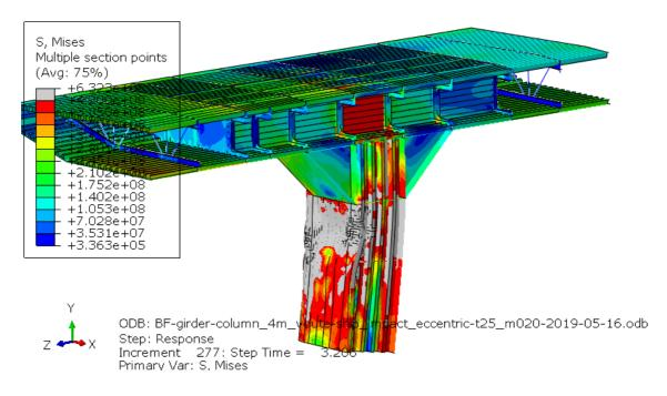
Figure 6-1 Plastic hinge in tall column (axis 3), local model. Local reinforcement of girder and a voute in the column top makes sure most plastic deformations takes place in the column. SeeAppendix F for details.
