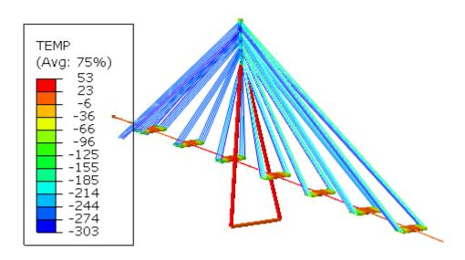
Figure 4-5 Post tensioning of cables and elongation of girder and tower with temperatures [K].
