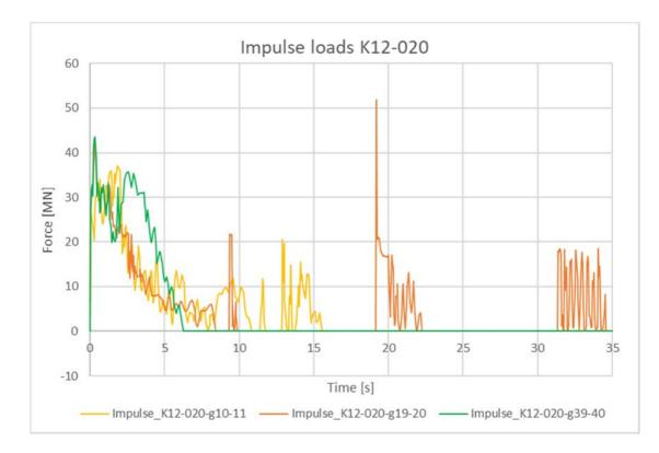
*Figure 5-2 Relevant impulse loads on bridge K12.*
