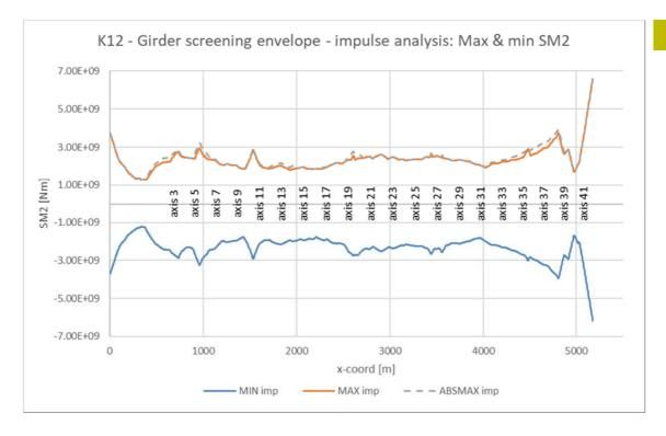
> Figure 5-3 Max and min envelopes for strong axis bending moments (SM2), [Nm]
