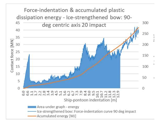
Figure 6-3 Force-indentation curve for pontoon impact with ice strengthened bulb.
