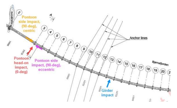
Figure 3-1 Ship impact illustration. Examples of the main impacts studied in this report.
