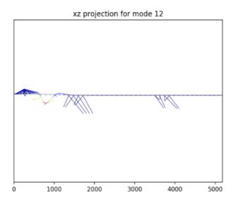
Figure 6-7 Mode 12 – pendulum mode of high bridge columns (model K12-020). From interactive and structural response analyses [11].
