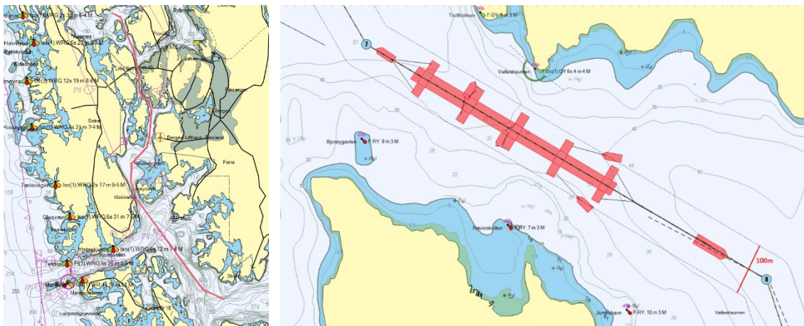
> Figure 8-8: Towing route (left) and towing of superelement through Vatløstraumen (right).
