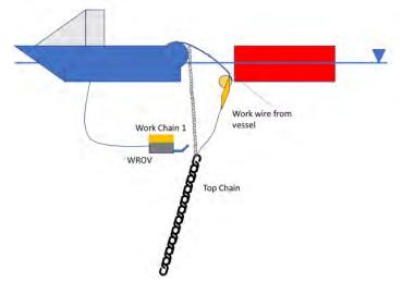
*Figure 9-16: Transfer of mooring line- step 3*
