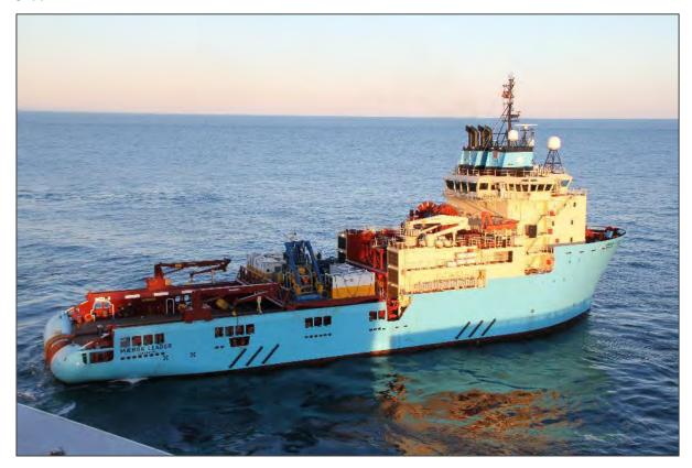
Figure 9-6 Example installation vessel Maersk Leader with two off temporary WROV systems
