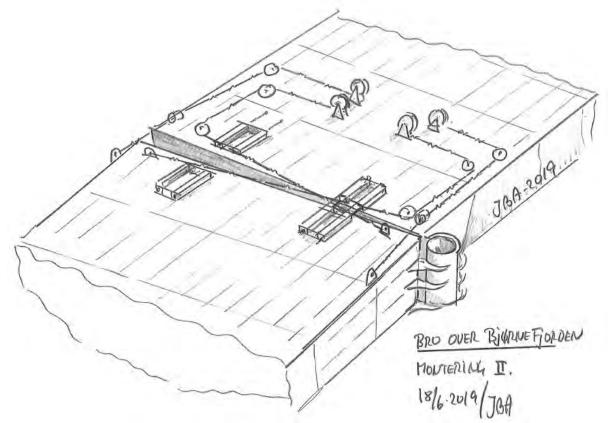
Figure 10-7 Bridge mating by guide joint - 1
