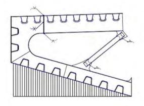
Figure 4-12 Assembly of top deck panel and truss brace
