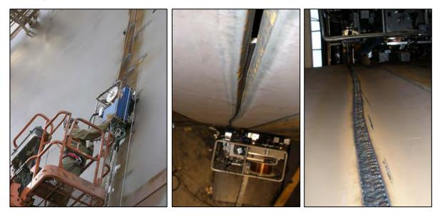
Figure 4-31 Self propelled and self positioning welding tractor for fully automated welding of section joints in the dock of OSS Lindø shipyard, using adaptive control to compensate for variations in groove position and gap
