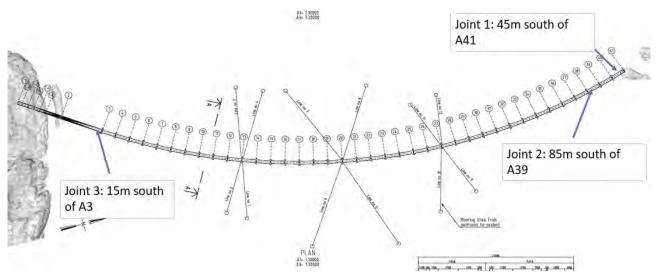
*Figure 10-4 Construction joints within deck box girder - 2 at north bridge end and 1 at south bridge end towards the cable stayed bridge*
