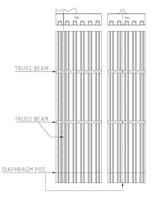
Figure 4-22 Panel fabrication for Section type 3
