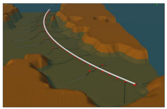
Figure 7-14: Mooring arrangement just prior to completion of bridge
