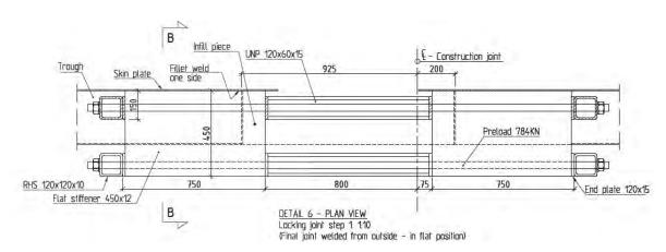
Figure 10-26 Locking joint for deck plate, construction joint 3 inclusive 800mm infill piece, longitudinal section
