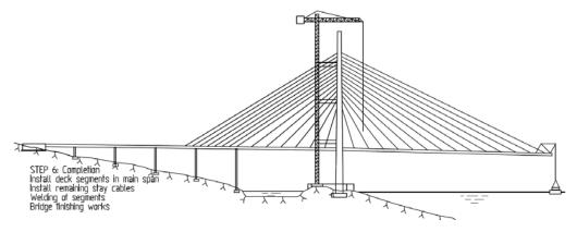
Figure 5-5 Construction of the main span deck
