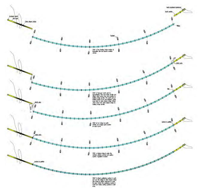
Figure 10-3: Installation of north section
