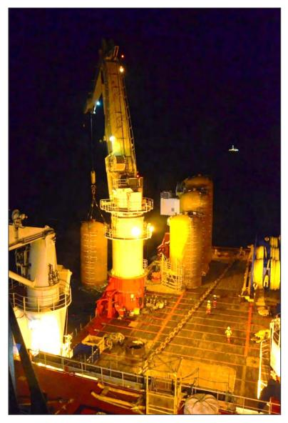
*Figure 9-5 Overboarding of suction anchor from BOA DeepC (250T crane). 152mm mooring chain running across deck. Wire-segments stored on reel drive system. (© Stefan Schlömilch)*
