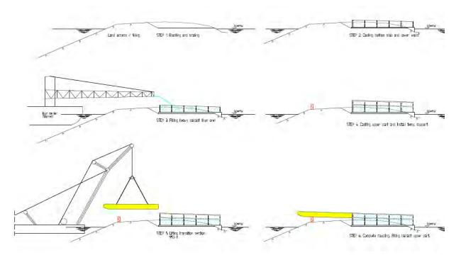
The floating bridge assembly will be performed on barges in a sheltered fjord (Søreidsvika). There bridge sections and pontoons with columns will be combined to form the floating bridge.
