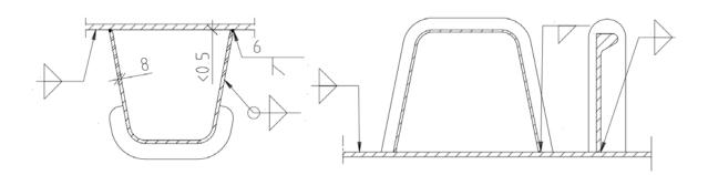
Figure 4-5 Welds between stiffeners, skin plate and T-beam
