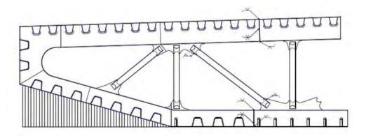
Figure 4-14 Assembly of complete "left half" of Bridge Girder
