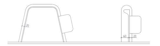
Figure 4-6 Welded-on plate pieces for stabilising stiffeners at transverse trusses
