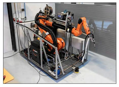
Figure 4-33 Mobile robotic welding unit (Inrotech)
