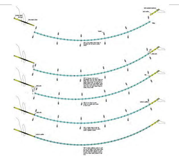
All installation operations are planned as weather restricted operations. The towing operations are planned to have a safe location in Bjørnafjorden, where the tow can survive a seasonal storm. The anchors are installed minimum one year before the bridge sections and mooring lines will be wet stored ready for hook-up when the bridge sections are installed
