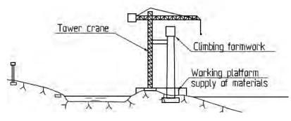
*Figure 5-1 Construction of tower*
