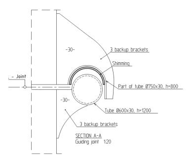
Figure 10-9 Guiding joint, plan view
