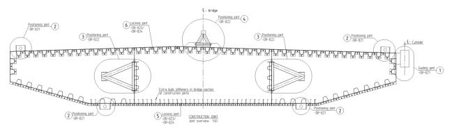
Figure 10-5 Cross section in bridge deck of floating bridge, 4.0 m deep and 27.0 m wide Guide joint (1), positioning joint (2)(3)(4), locking joint (5)(6)
