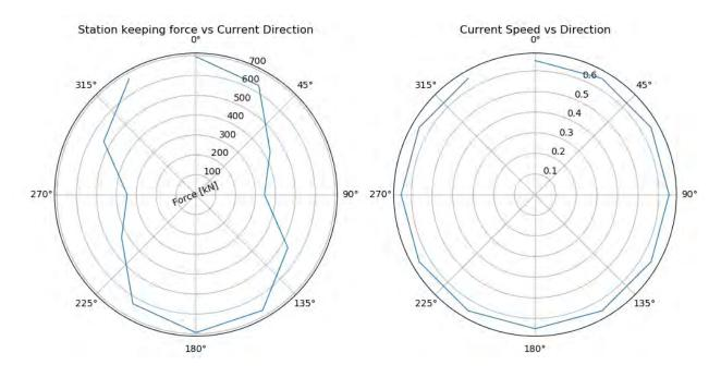
*Figure 7-16: Forces acting on the bridge due to current. (Current towards north = 0 deg). Omnidirectional assumptions.*
