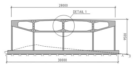
*Figure 6-6: South abutment elevation view*
