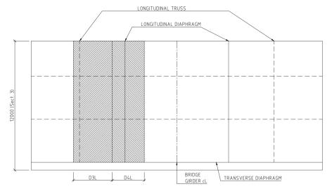
Figure 4-20 Plan of special deck plate section 3
