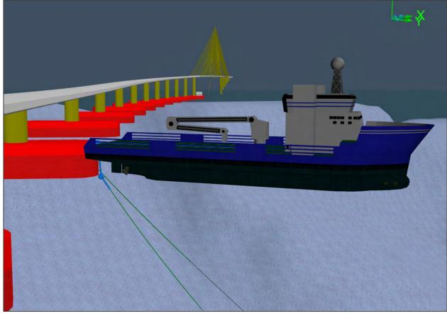
*Figure 9-19: Mooring line tensioning at pontoon with bumper. Only very low thrust forces are needed in this configuration.*
