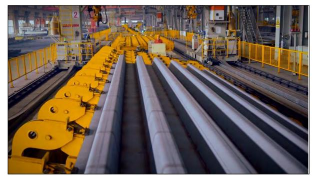
Figure 4-40 Deck panel with troughs on fixture, in China
