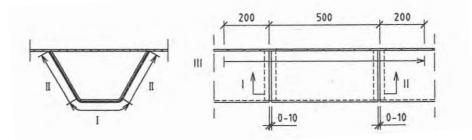
Figure 4-23 Welding details for in-fill member for U-rib (numbers denote weld sequence)
