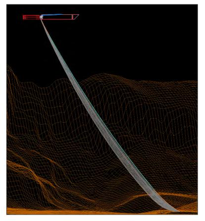
*Figure 9-22: Overview/Time trace of tensioning process when tensioning at pontoon*
