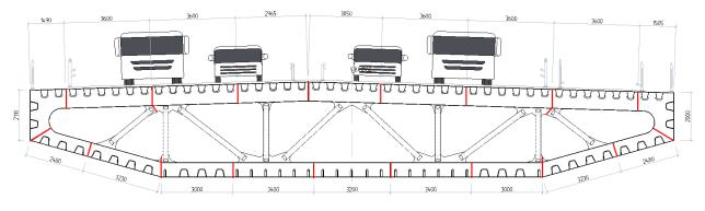
Figure 4-4 Sectioning in transverse direction
