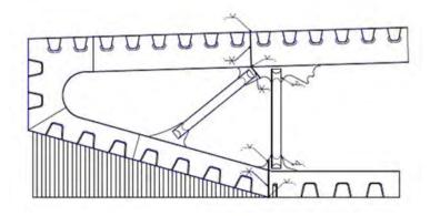
Figure 4-13 Assembly of top and bottom deck panels together with truss column
