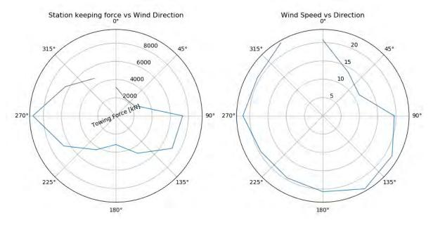
Figure 7-15: Forces acting on the bridge due to wind. (Wind from north = 0 deg)
