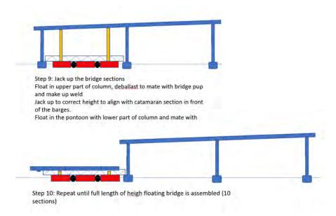
Figure 7-11: High floating assembly sequence – 3
