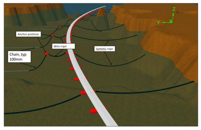
Figure 7-13: Typical moorings system layout
