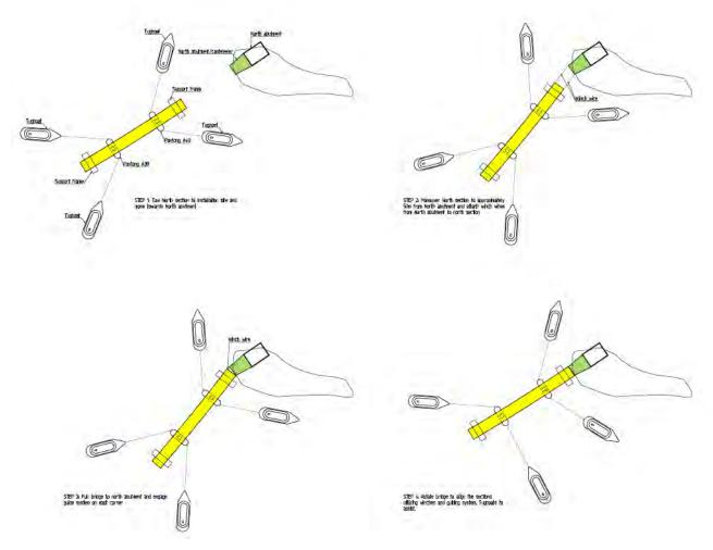
Figure 10-2: Installation of north section
