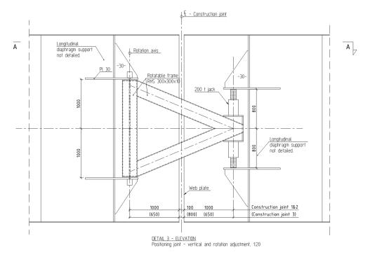
Figure 10-13 Positioning joint, vertical direction, elevation
