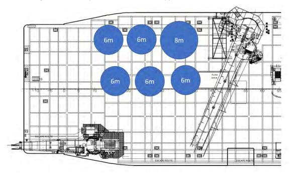
*Figure 9-3: Deck Layout of typical installation vessel*
