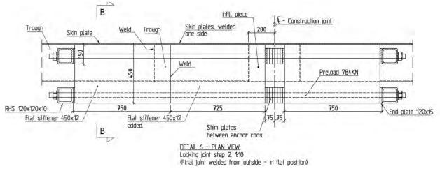
Figure 10-27 Locking joint for deck plate, construction joint 3 inclusive 800mm infill piece, longitudinal section Infill skin and stiffener plates now welded into position
