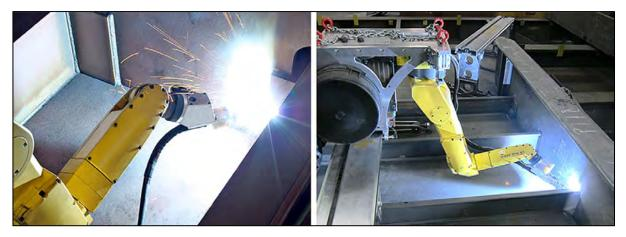
*Figure 4-32 Robotic welding between webs, stiffeners and deck plate. The robot identifies the structure and welds automatically. (Source: Inrotech)*
