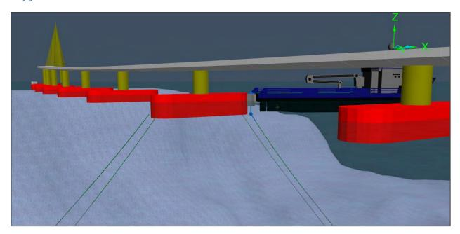
*Figure 9-20: Mooring line tensioning at pontoon with bumper. Only very low thrust forces are needed in this configuration.*
