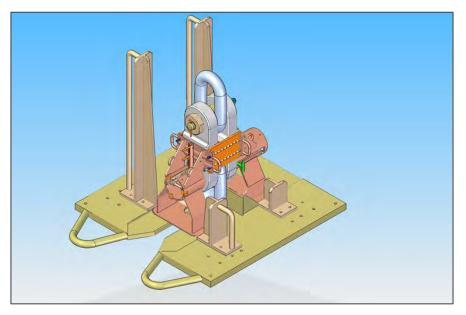
*Figure 9-8 H-shackle with ROV kit during connection to chain supported on anchor hang-off table (illustration by Vicinay)*
