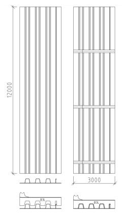
Figure 4-8 Assembly of bottom panel
