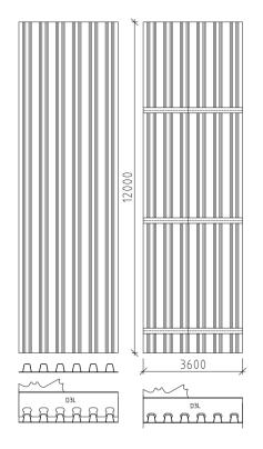
Figure 4-7 Assembly of deck panel
