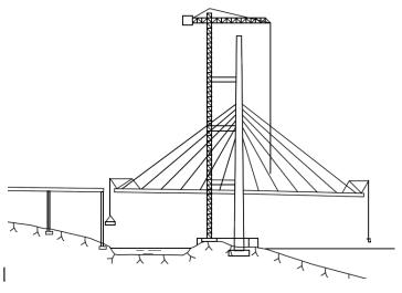
Figure 5-4 Cantilever construction
