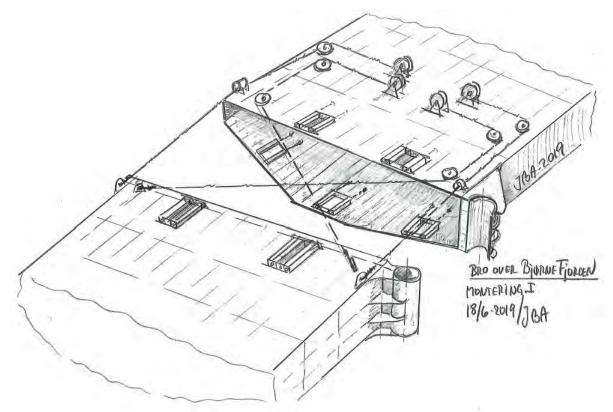
Figure 10-6 Bridge mating by guide joint - 1
