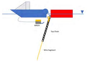
*Figure 9-18: Transfer of mooring line- step 5*
