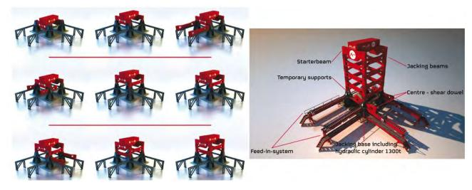
Figure 7-8: Jacking towers principle
