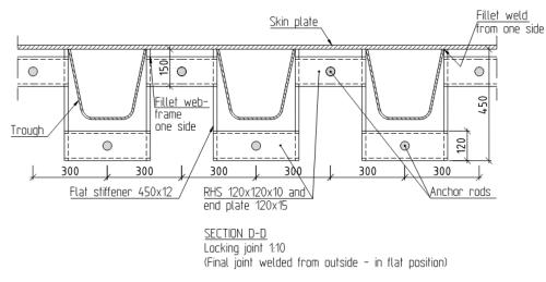
Figure 10-23 Locking joint for deck plate, construction joint 1 & 2, transverse section
