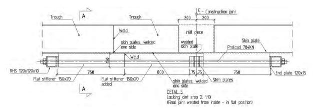
*Figure 10-25 Locking joint for web- and bottom plates, construction joint 3 inclusive 800mm infill piece, longitudinal section Infill skin and stiffener plates now welded into position*
