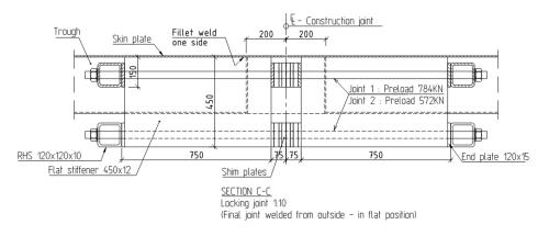
Figure 10-22 Locking joint for deck plate, construction joint 1 & 2, longitudinal section
