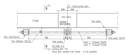
Figure 10-19 Locking joint for web- and bottom plates, construction joint 1 & 2, longitudinal section
