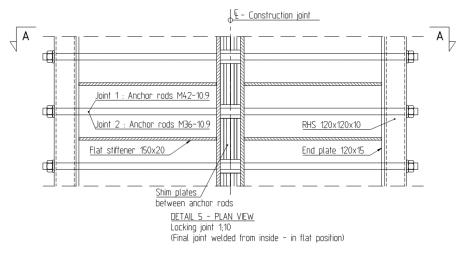
Figure 10-18 Locking joint for web- and bottom plates, construction joint 1 & 2, plan view
