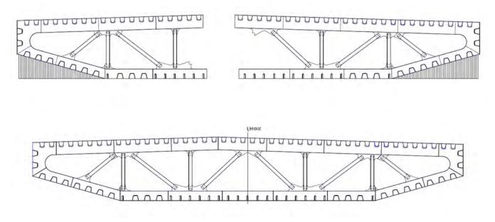
Figure 4-15 Assembly of entire Bridge Girder including back-welding
