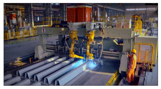
Figure 4-39 Robotic welding gantry in China. Process could be metal cored wire welding, or possibly MAG/CAW
