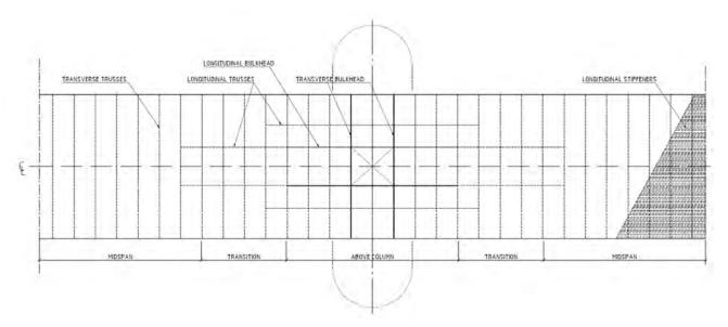
Figure 4-2 Overview of longitudinal trusses and bulkheads
