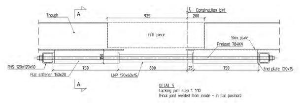
*Figure 10-24 Locking joint for web- and bottom plates, construction joint 3 inclusive 800mm infill piece, longitudinal section*
