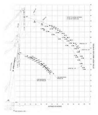
Figure 6-4 Crane curve Taklift4 (© Boskalis)
