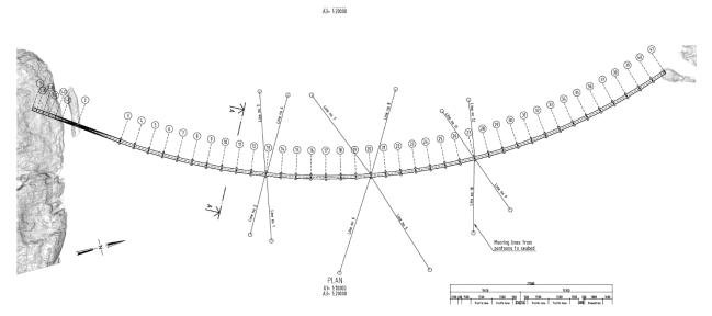
*Figure 9-1 Principle mooring line arrangement*
