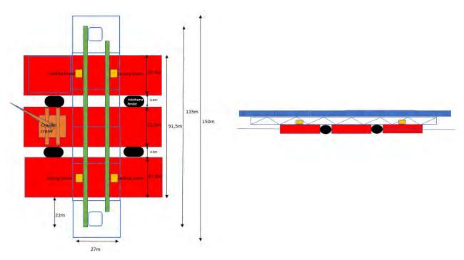
Figure 7-4: High floating bridge assembly site set up
