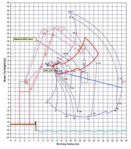
*Figure 9-4: Crane chart of typical 400T crane*
