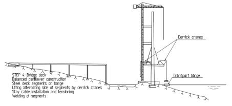
*Figure 5-3 Installation of the first cable stays*
