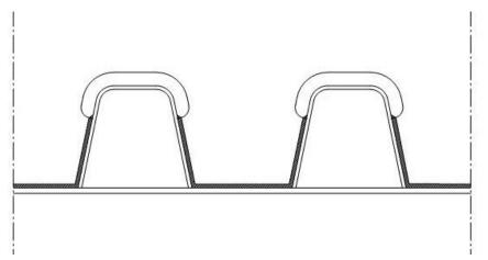
Figure 4-35 Fillet welds between diaphragms/stiffeners, troughs and deck are an obvious case for robotic welding
