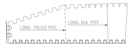
Figure 4-21 Section 3 transverse diaphragm assembly
