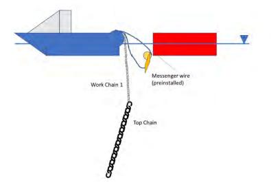
Figure 9-15: Transfer of mooring line- step 2
