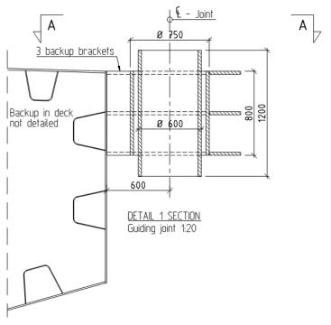
*Figure 10-8 Guiding joint, section in construction joint*
