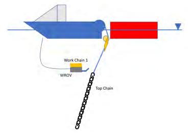
Figure 9-17: Transfer of mooring line- step 4
