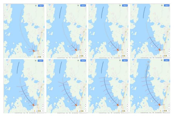
Figure 7-12: Low floating assembly and mooring process
