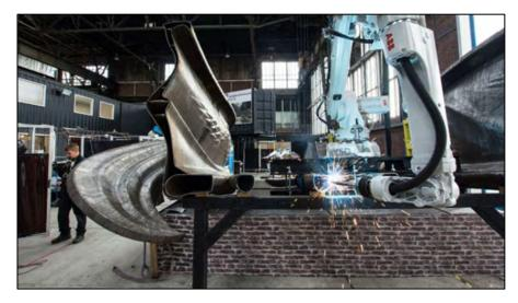
*Figure 4-29 Welding robot in action during 3-D printing of bridge. MX3D project, Amsterdam*
