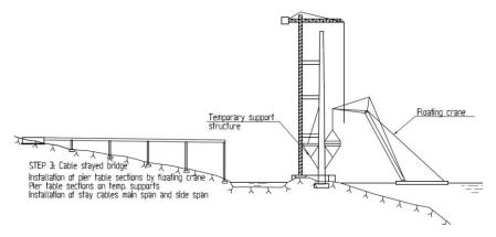
Figure 5-2 Installation of the two first sections to tower
