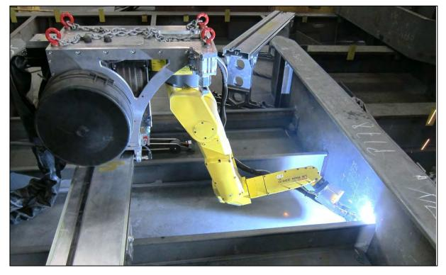
*Figure 4-36 Robotic welding concept which might also be used for fillet welds between diaphragms/stiffeners, troughs and deck*
