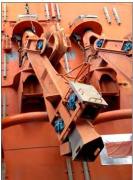
Figure 9-13: Dual axis fairlead with chain stopper (©Flint-tech and MacGregor Pusnes)
