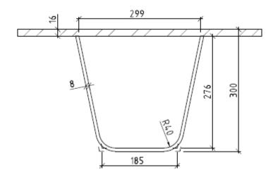
Figure 10-28 Deck and trough configuration used in
