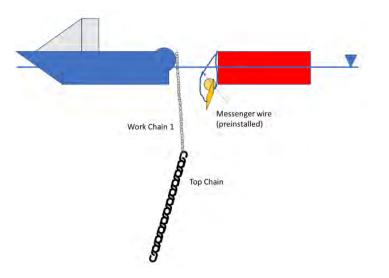
Figure 9-14: Transfer of mooring line- step 1
