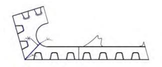
Figure 4-10 Assembly of web panel to the two inclined bottom panels
