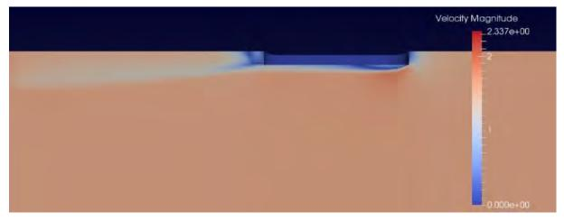
*Figure 2-10 Velocity fields for pontoon in steady flow seen in a centre-cut parallel with the pontoons length axis.*
