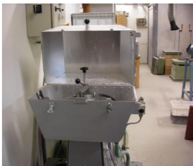
Figur 10.4 Prall-test (Foto: SINTEF)
