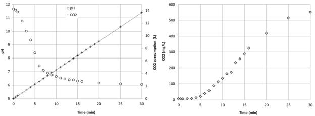
**Figure 6.** Tunnelling waste water from Gran at 10 °C. Plot of pH and CO<sub>2</sub> concentration versus time after addition of CO<sub>2</sub> gas started. The straight line represents accumulated consumption of CO<sub>2</sub>.
