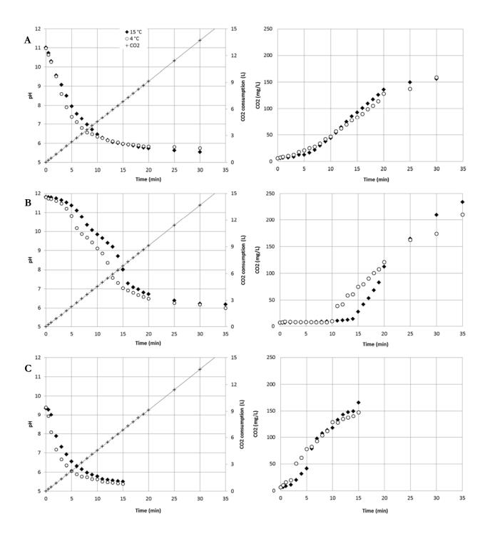
**Figure 4.** Average results from two replicate experiments with synthetic solutions at 4 and 15 °C. The difference between replicates was small and not indicated in the plots. The panels show pH (left) and  $CO_2$  concentration (right) versus time after addition of  $CO_2$  gas started for the experiment with **A** Tap water adjusted to pH 11, **B** "Lofast" water, and **C** "Frodeåsen" water. The straight lines represent accumulated consumption of  $CO_2$ .
