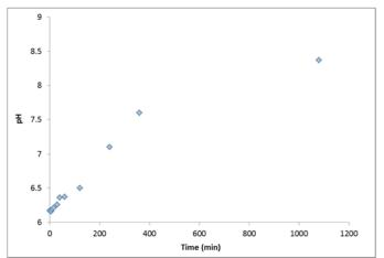
Figure 5. pH as a function of time for synthetic Lofast water at 15 °C as CO<sub>2</sub> is degassing
