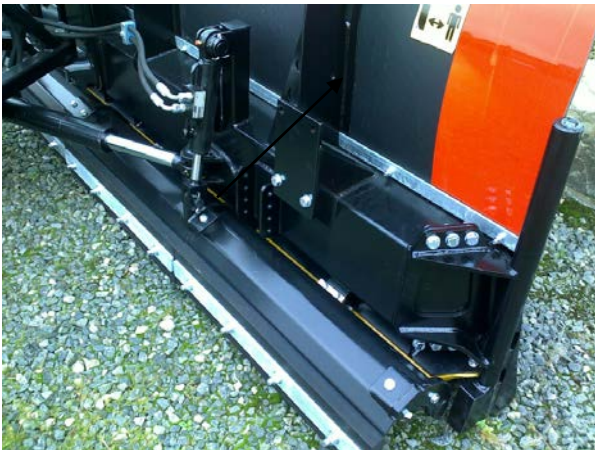
Figur 4-19 Hydraulisk betjente slapseelementer (kilde: Arctic Machine)
