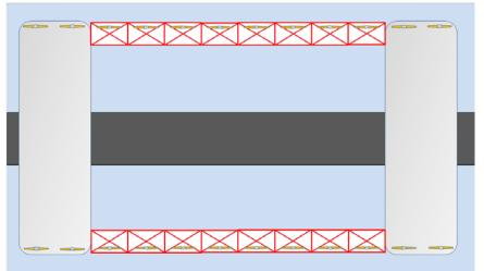
*Figure 20* Concept for using truss structures to allow for additional rows of TISEC devices in the downstream direction for a floating bridge (seen from below).
