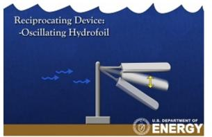
*Figure 5 Oscillating hydrofoil design principle [18].*
