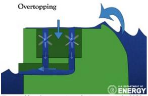
Figure 12 Overtopping design principle [18].
