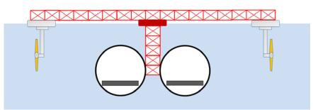
Figure 23 Concept for using truss structures and pontoons to allow for additional rows of TISEC devices in the downstream direction for a submerged floating (seen from the side).
