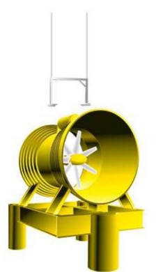
Figure 6 Enclosed tips (Venturi) design principle [19].
