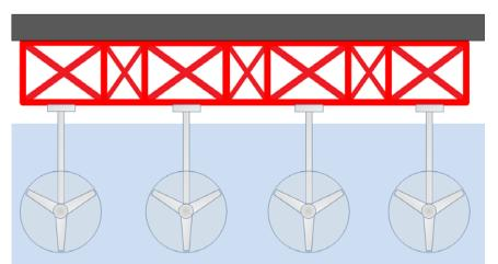
Figure 25 Concept for using truss structures to increase the number of TISEC devices that can be utilized for a suspension bridge.
