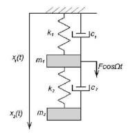
**FWEPS dynamic model:** The oscillating system consists of a capsulefloat able to oscillate in water and an elastic pendulum with a large mass weight suspended inside. The system can be simulated adequate enough by a two-degree-of-freedom oscillating model (see scheme).
