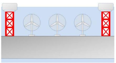
*Figure 24* Sketch showing how the number of TISEC devices in the cross-stream direction can be limited by additional structures for a submerged floating tunnel.
