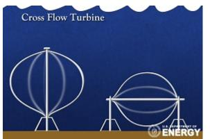
*Figure 4* Cross-axis or cross flow turbine design principle [18].
