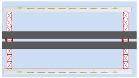
Figure 22 Concept for using truss structures and pontoons to allow for additional rows of TISEC devices in the downstream direction for a submerged floating tunnel (seen from below).
