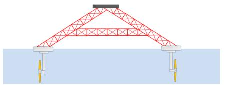
Figure 19 Concept for using truss structures and pontoons to allow for additional rows of TISEC devices in the downstream direction for a suspension bridge (seen from the side).
