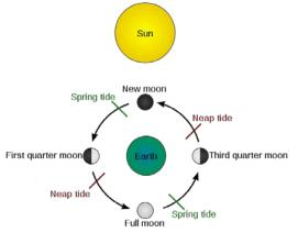
Figure 1 Tidal variation schematic.
