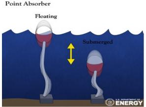
*Figure 9 Floating point absorber and submerged pressure differential design principles [18].*
