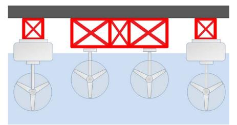
Figure 26 Concept for using truss structures to increase the number of TISEC devices that can be utilized for a floating bridge.
