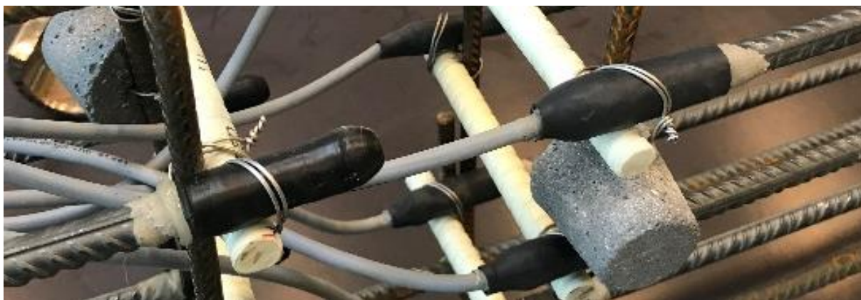
Figure 2-3. Photo of coated ends on working electrodes.
