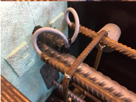
Figure 3.3. Photographic documentation of epoxy treatment of electrical contact between rebar cage and cables.
