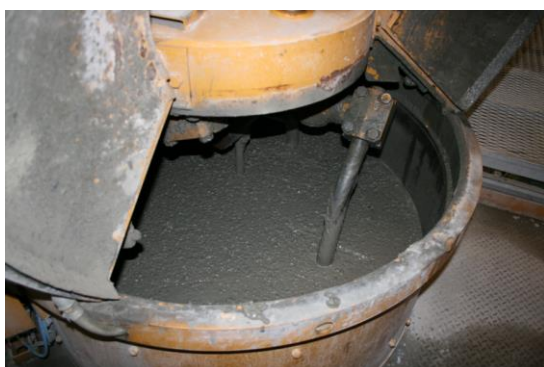
Figure 2.4. To the left a view into the Haarup 375/250 litre concrete mixer. To the right the vibration during casting of a concrete element is seen.
