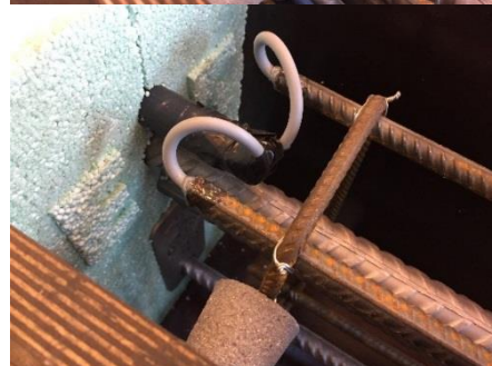
Figure 3.3. Photographic documentation of epoxy treatment of electrical contact between rebar cage and cables.
