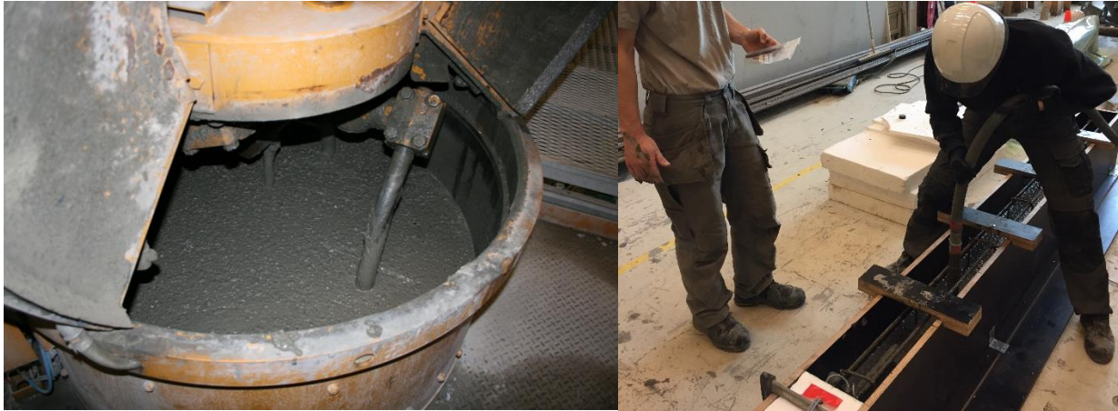
Figure 2.7. Left: A view into the Haarup 375/250 litre concrete mixer. Right: The vibration during casting of a concrete element is shown.
