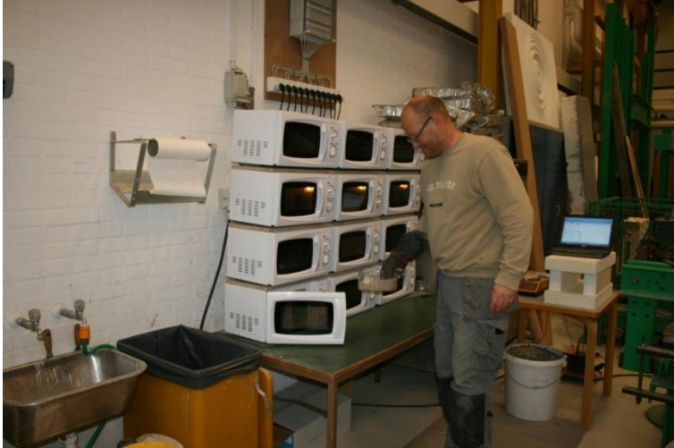
Figure 2.6. Microwave ovens used to determine the moisture content of aggregate fractions.
