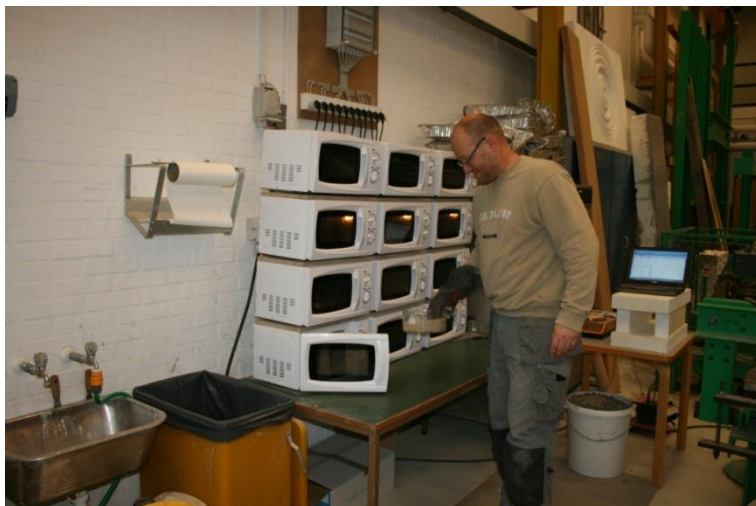
Figure 2.3. Microwave ovens used to determine the moisture content of aggregate fractions.
