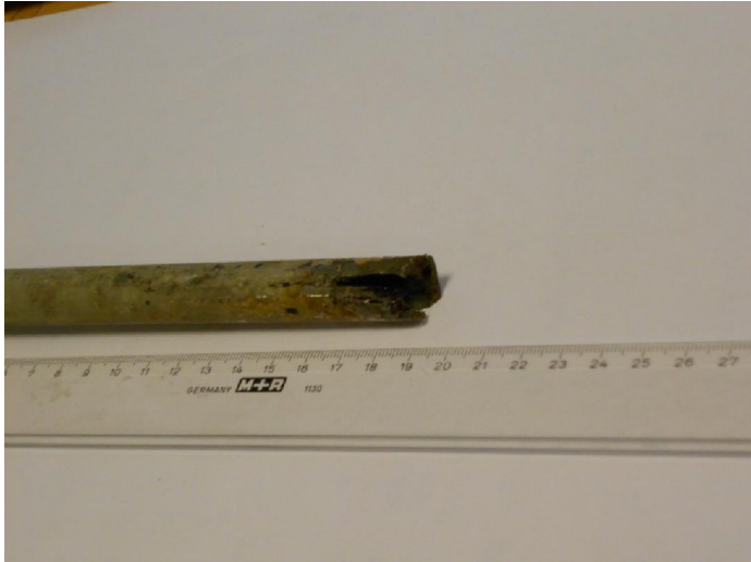
Figure 2. Stainless steel bolt. The hollow corroded end.
