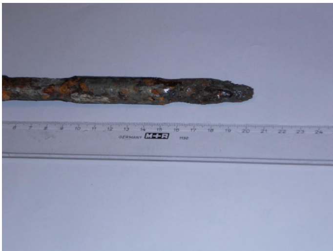
Figure 1. Stainless steel bolt. The pointed corroded end.
