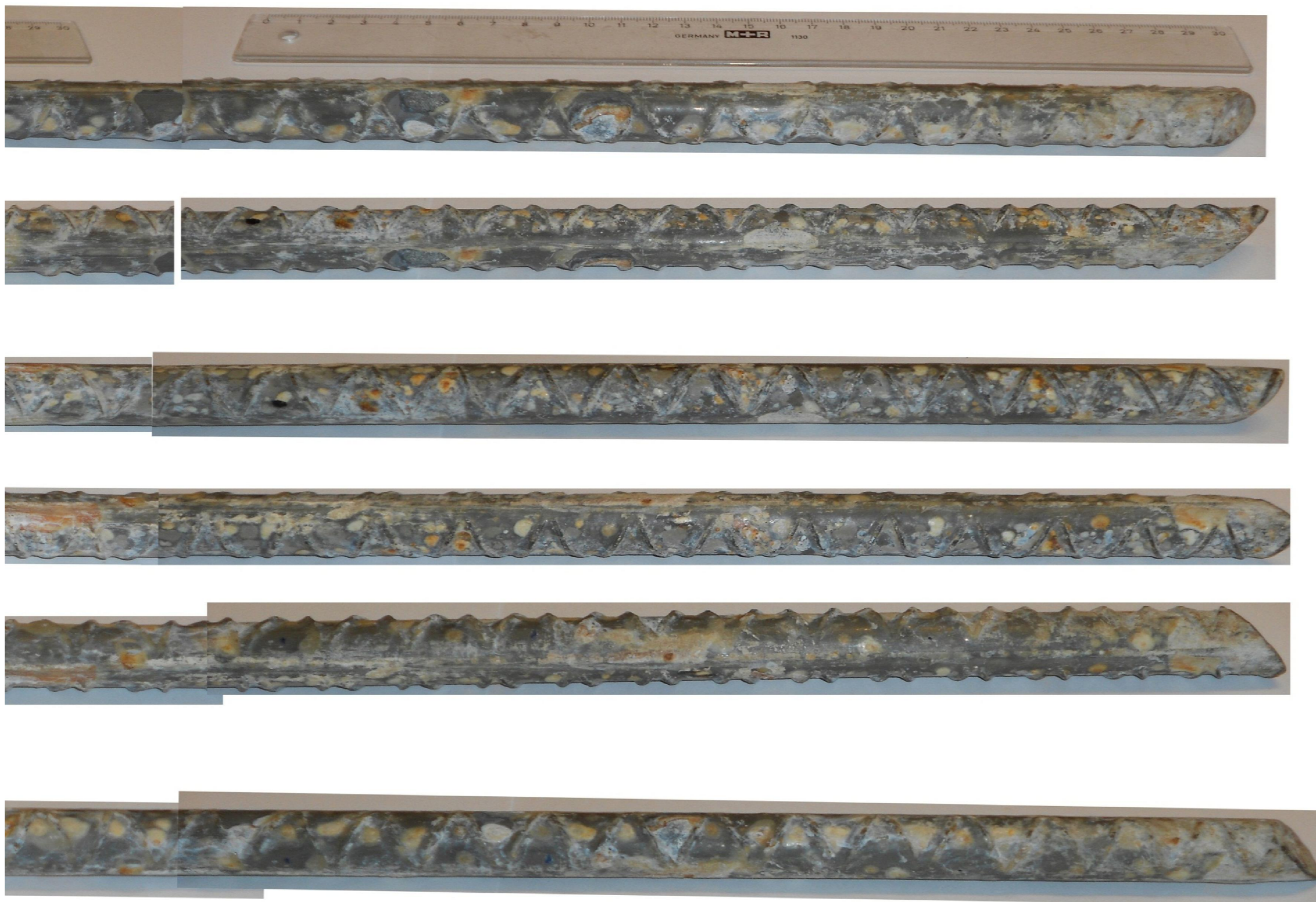
Figure 10. Bolt nr. 5 Galvanized with one layer of clear epoxy after cleaning.
