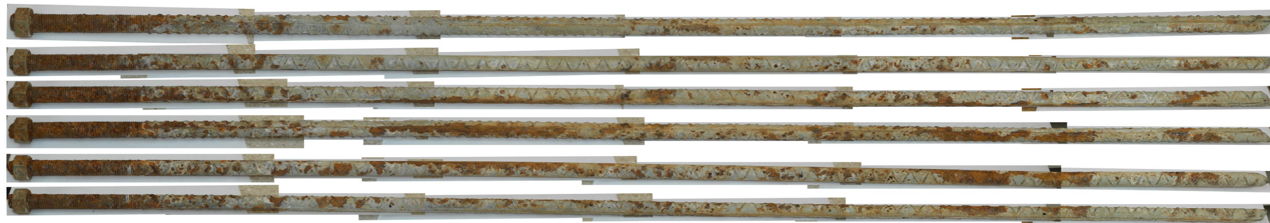
Figure 7. Bolt nr. 5 Galvanized with one layer of clear epoxy before cleaning.
