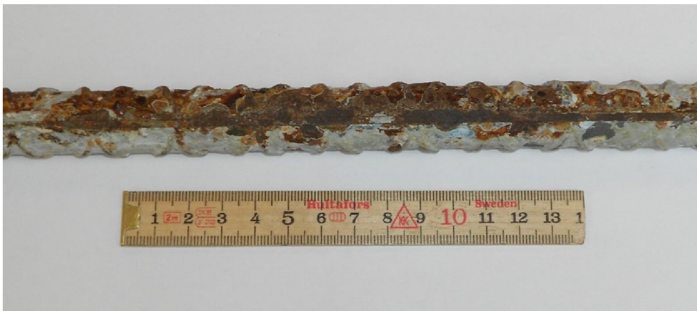
Figure 5. Bolt nr. 6. Surface corrosion and pitting.
