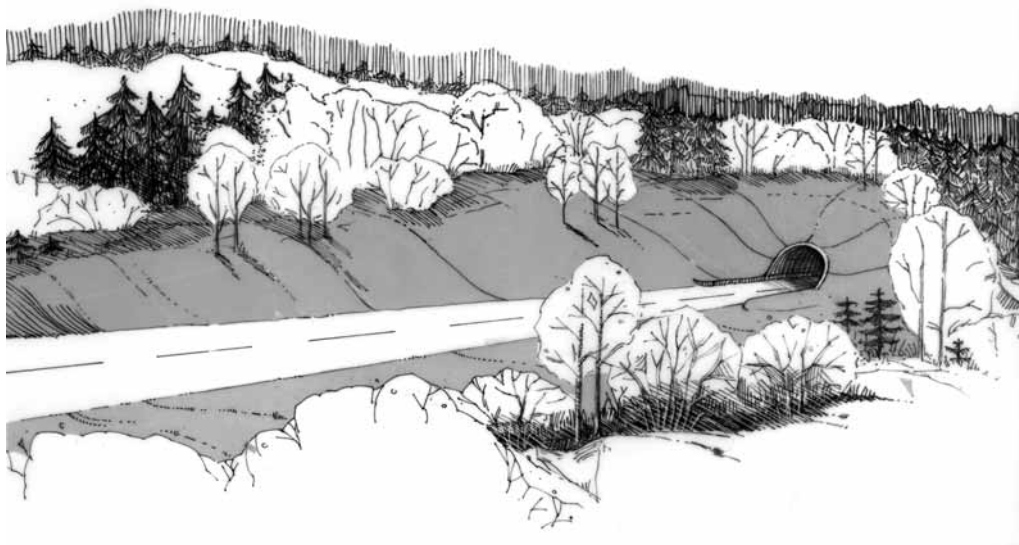
Figure 5.4 Approach zone in an area with slight gradient. In order to avoid the impression of entering a shaft at the tunnel entrance, the landscape has been comprehensively planned. Illus. Ingeborg Langeland Degnes.
