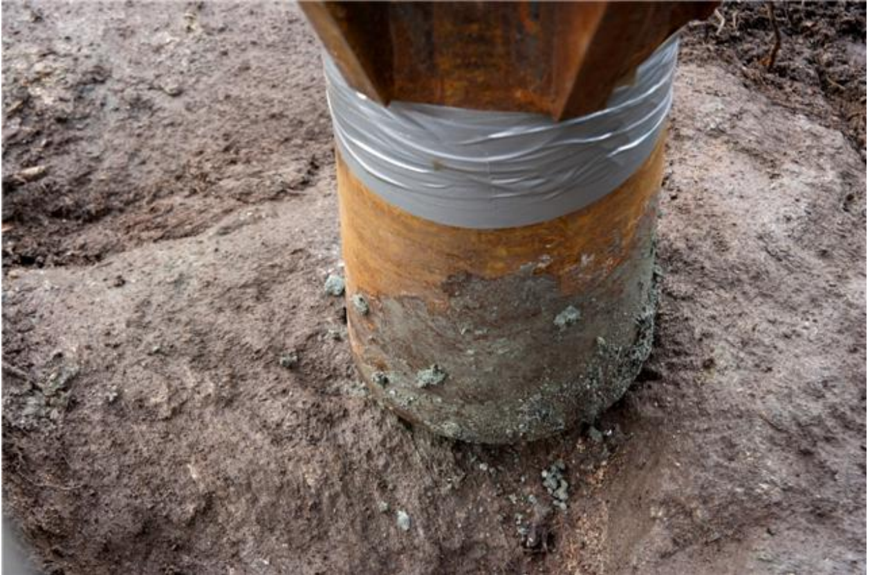
The rock surface before the shoe was driven.
