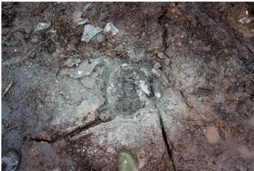
Figure 5-11: Photos of the rock in various stages before and after driving shoe no. 3.
