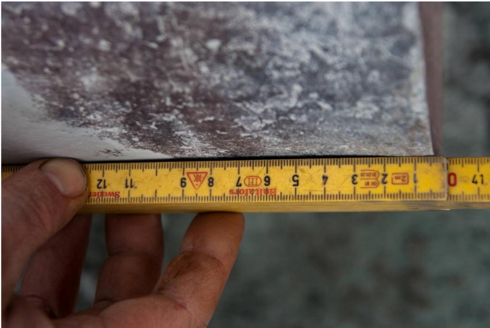
Plastic deformation of NPRA shoe 1
