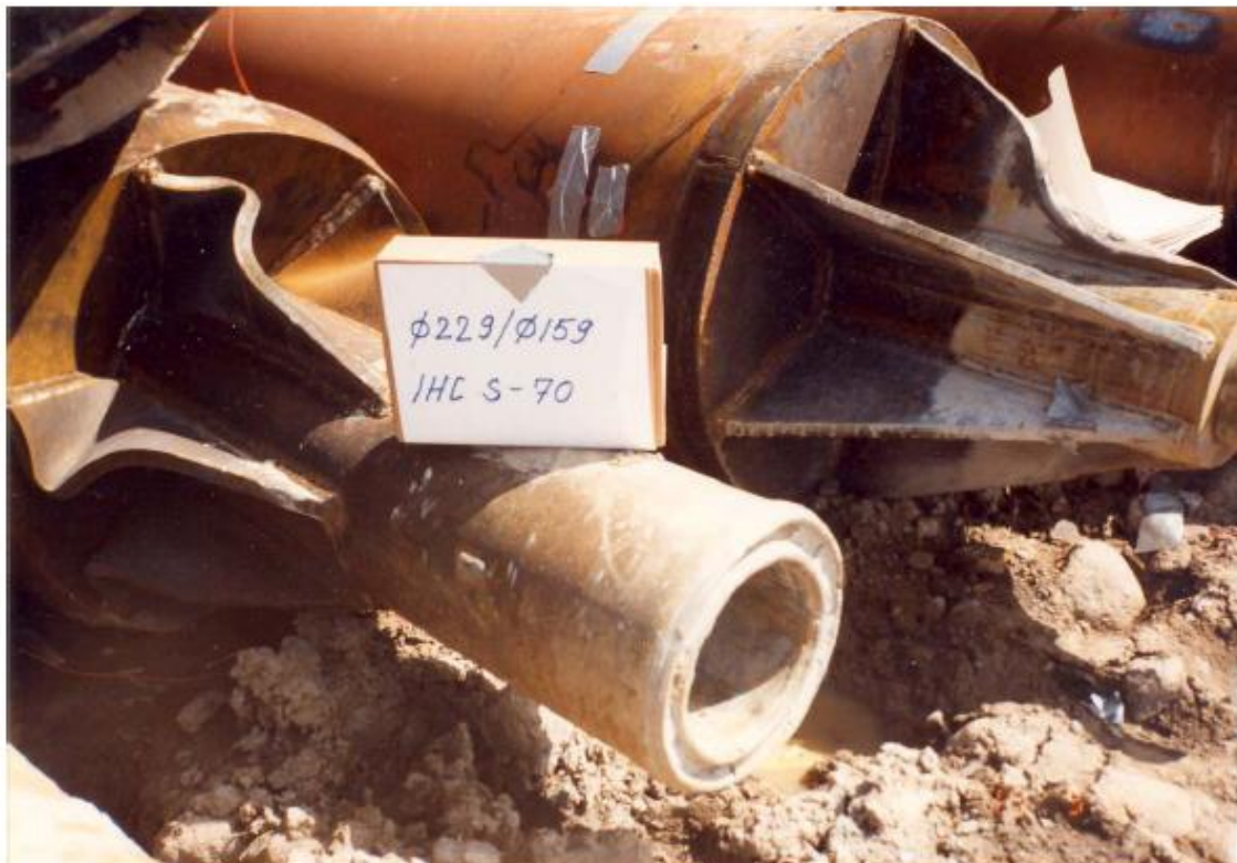
Figure 9-2: Buckling of the stiffening plates with thickness t = 15 mm Photo: Hannu Jokiniemi.
