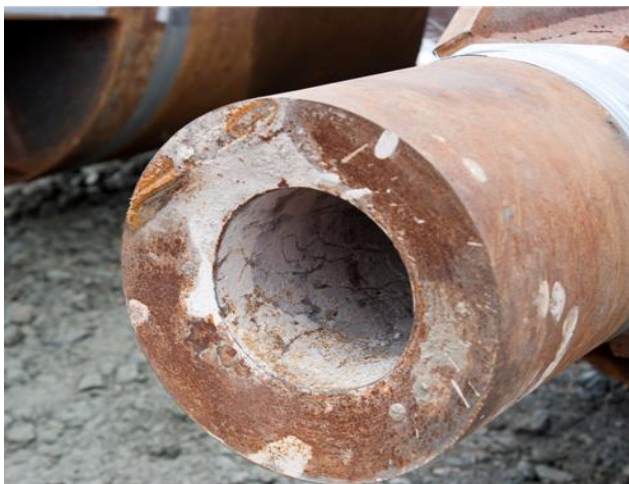
Hardened shoe no. 1 and 2 with concave end-face
