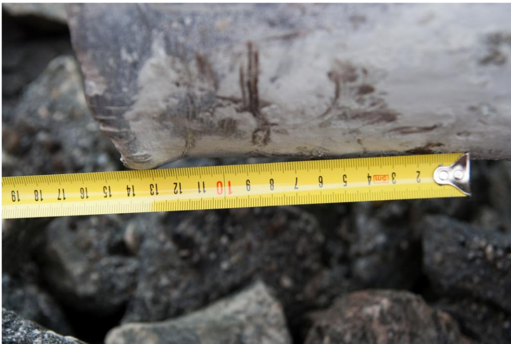
Plastic deformation of NPRA shoe 2
