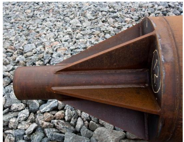
Shoe no. 3 has a base plate thickness of 70 mm
