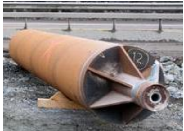
Shoe no. 3 with shoe area 0.037 \text{ m}^2
