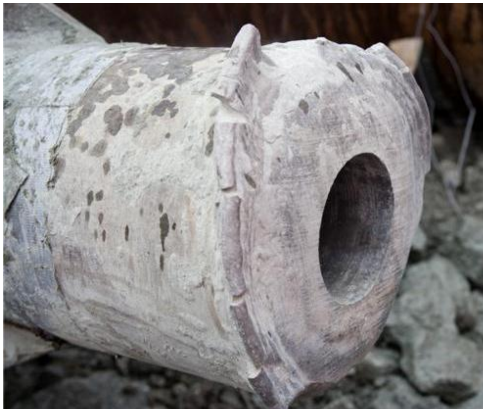
Lower edge of shoe surface after the shoe was driven.
