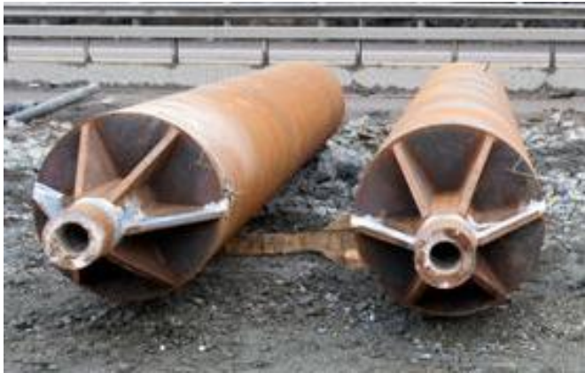
Shoe no. 1 and 2 with shoe area 0.027 \text{ m}^2
