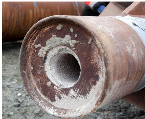
Shoe no. 3 with build-up weld on flat end
