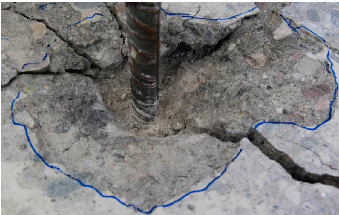
Figure 7-10: Crater made by the straight shoe with predrilling, test series 4
