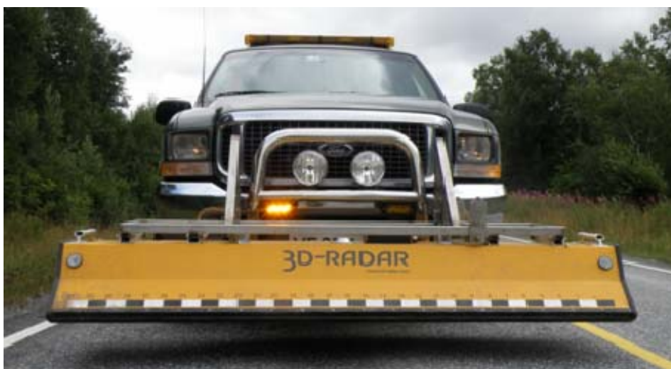
Figur 4.9 3D-GPR (3-Dimensional Ground Penetrating Radar). (Foto: SINTEF)
