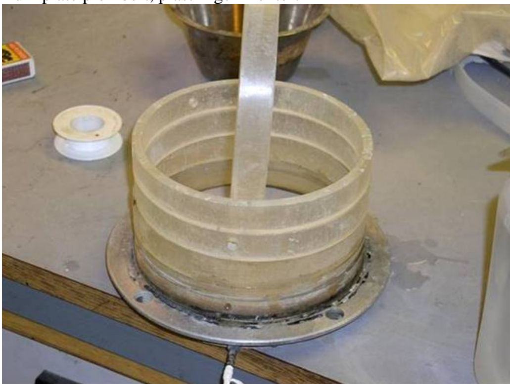
Bunnplate plombert, plastringer montert
