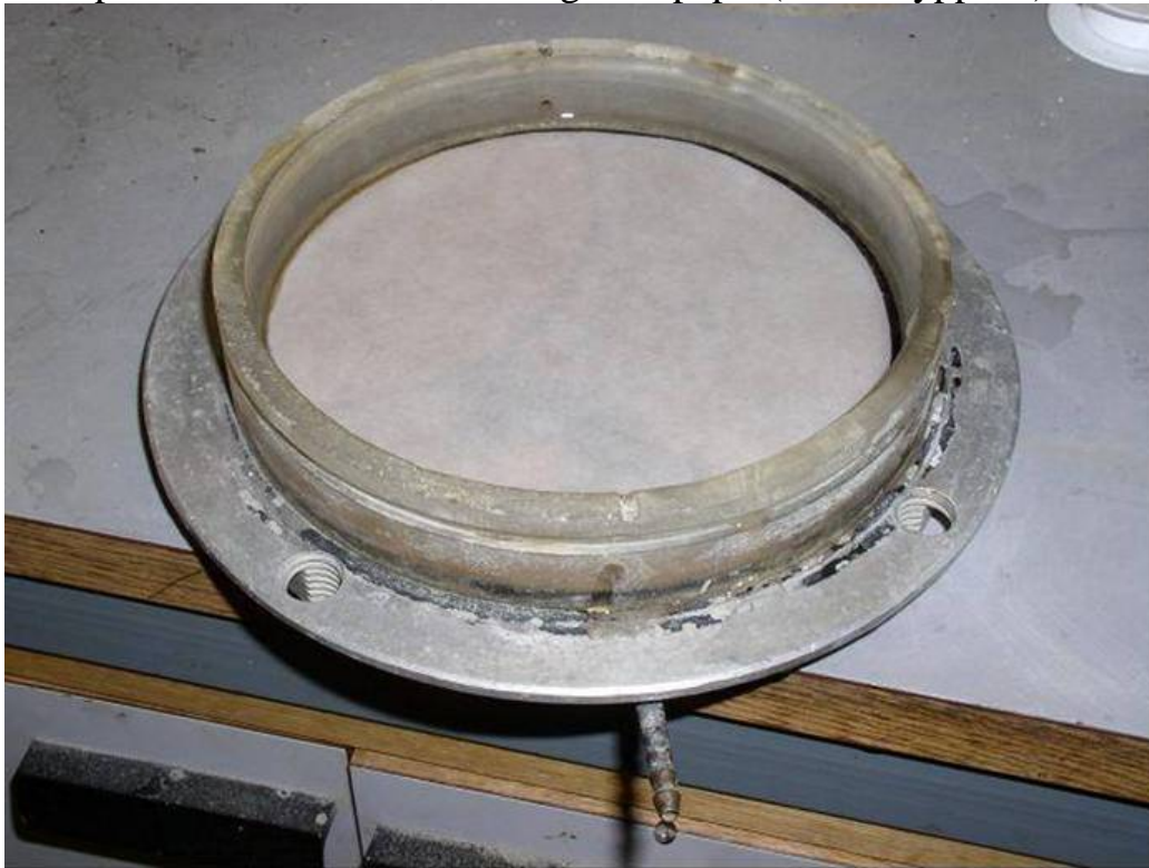
Bunnplate plombert, plastringer montert
