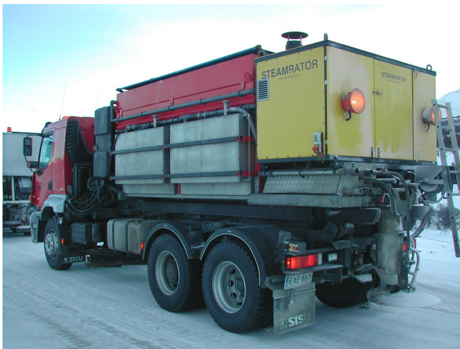
Figur 2.7: Fastsandspreder fra Arctic Machine, NCC Finland
