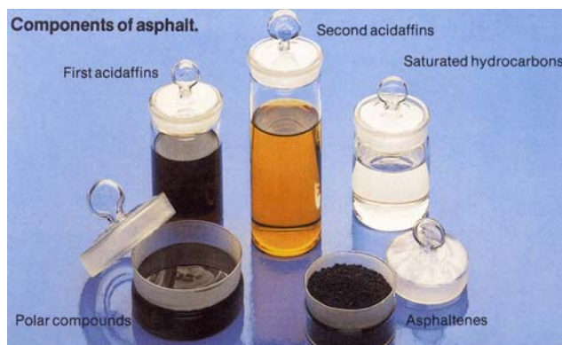
Asphalt Binder Fractions, Asphaltenes and Maltenes.
