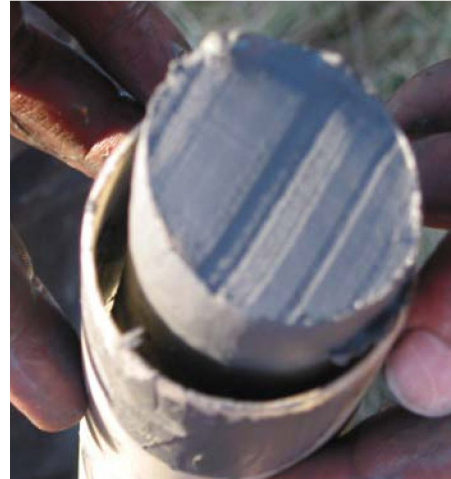
Figure 10 Strain in sample more than 2 x diameter
