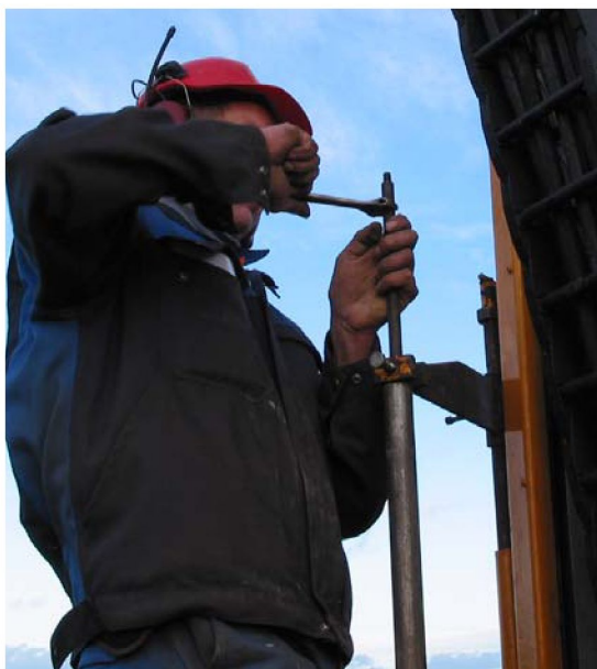
Figure 5 "gallows" for fixation of piston rod – Multiconsut
