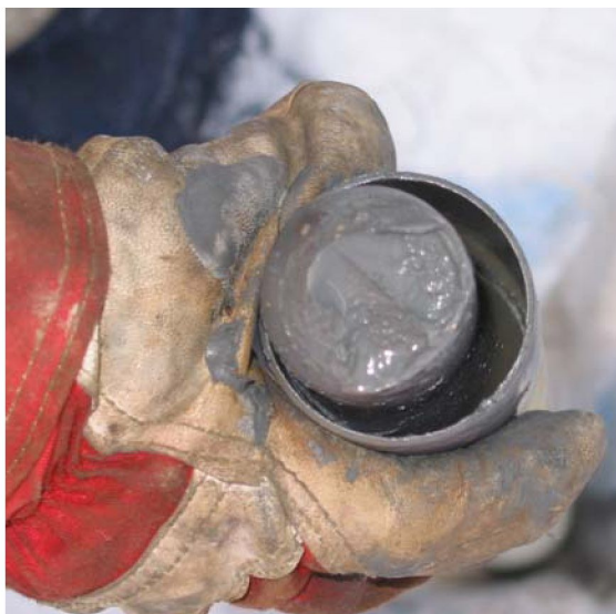
Figure 19 Maximum tensional sample strain observed - 2 x diameter
