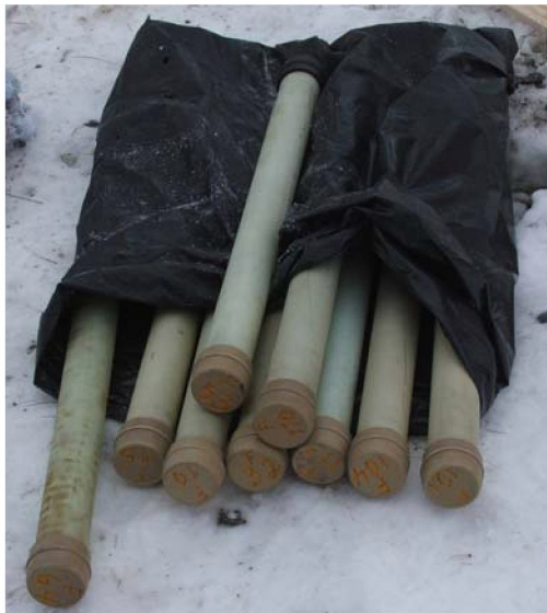
Figure 17 Cleaned cylinders with sealing cups mounted
