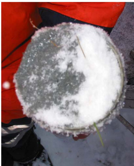
Figure 15 The sample end was put on snow before sealing
