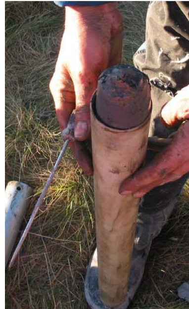
Figure 8 Use of screwdriver for cutting sample flush with cylinder end
