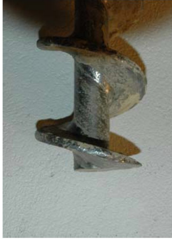
Figure 21 Modified auger with flat and sharp end for predrilling to sampling level
