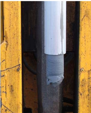
Figure 9 Sampler in rig without cutting edge
