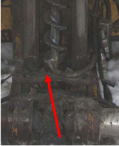
Figure 21 Modified auger with flat and sharp end for predrilling to sampling level
