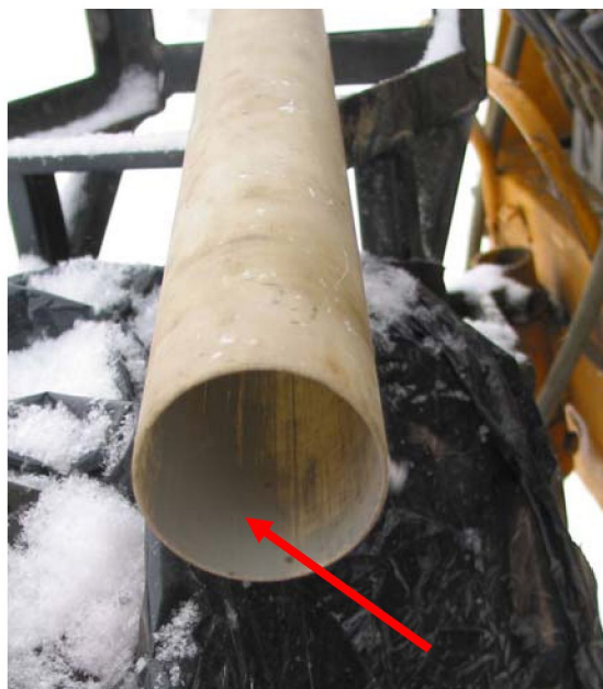
Figure 11 Clay residue in cylinder
