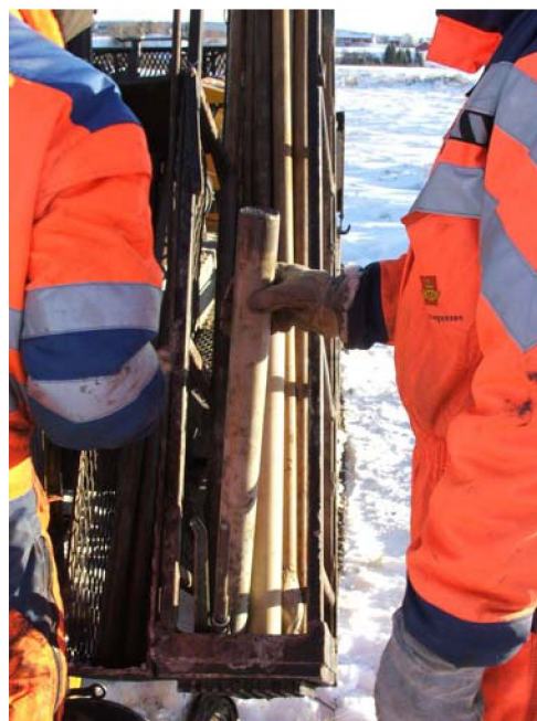
Figure 16 Storage of sample cylinders in the drill rod storage box with engine running
