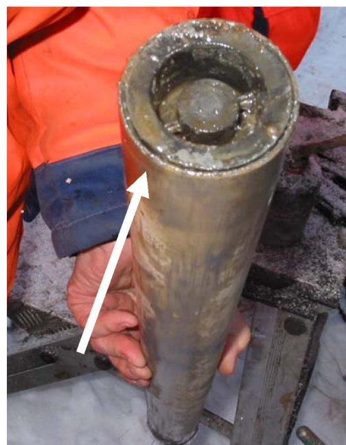
Figure14 Piston drawn out of the cylinder during release from sampler.
