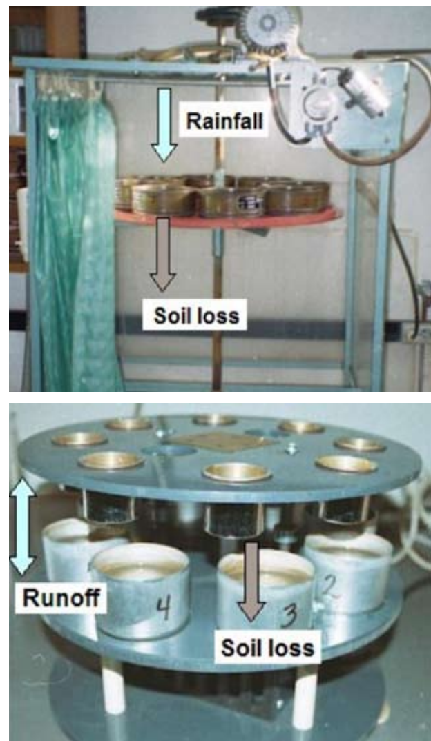
Figure 4. Rainfall simulator (top), where water drops fall from nozzles onto the sieves with aggregates, and wet-sieving apparatus (bottom) where sieves with aggregates are raised and lowered into water-filled containers to simulate runoff.
