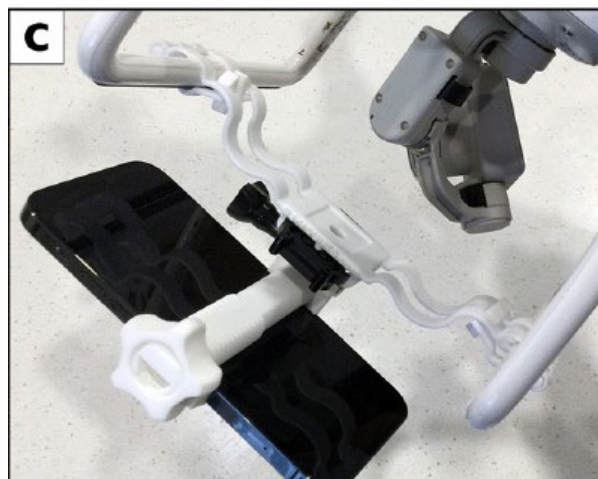
Figure 4. iPhone on a Commercial UAS used for Snow Depth Measurement (King et al. 2023).
