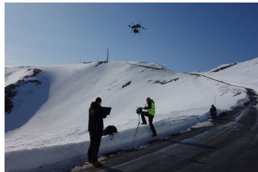
Figure 3. A UAS Carrying Ground Penetrating Radar During the 2018 Test at Andøya
