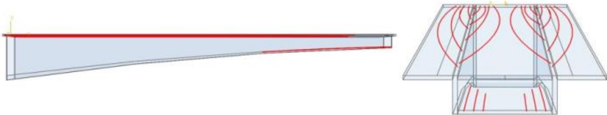
Figure 18: PT tendons in numerical model
