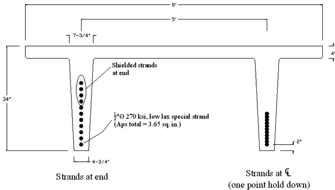
**ID-9.2.** Double-T beam cross-section (Poston and West, 2005).
