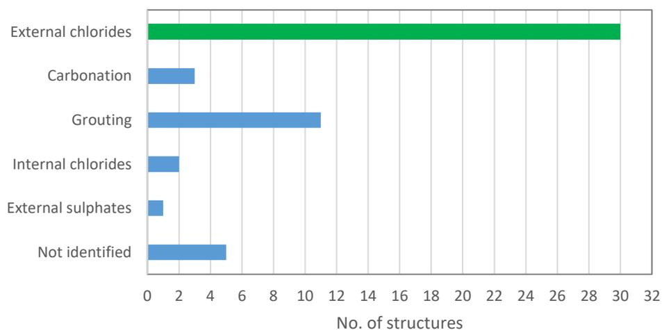
**Figure 4.2.1.** Major corrosion causes of the studied structures.
