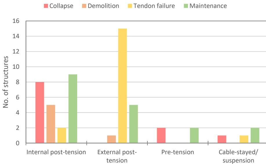
**Figure 3.1.3.** Level of damage in the studied structures divided by type of prestressing system.
