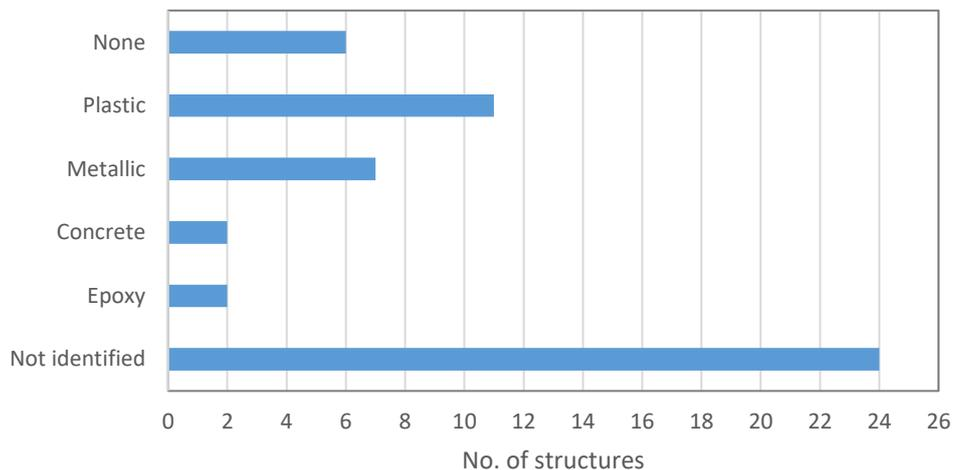
**Figure 2.3.1.** Type of ducts in the studied structures.
