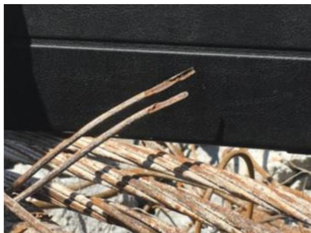
**ID-6.8.** Pit corrosion in the debris after failure (Nutti et al, 2020).
