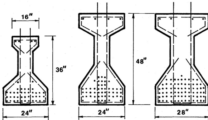
**ID-32.1.** Typical bridge girder sections used on Illinois Tollway bridges (Gustafarro et al, 1983).
