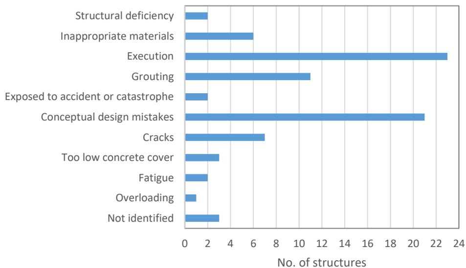
**Figure 4.1.1.** Major failure causes of the studied structures.
