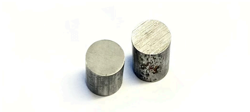
Figure D.9: Left sample: with oxide layer. Right sample: without oxide layer.
