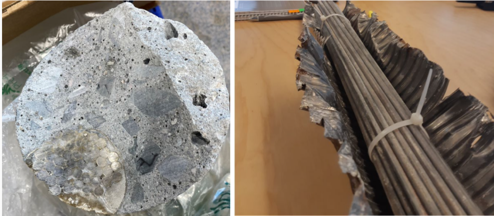
Figure 5.1: Test materials from Farriseide bridge. Left: A section of concrete extracted, containing a tendon duct with tensile wires embedded in grout. Right: Tendon duct and tensile wires after removal of concrete and grout [50].
