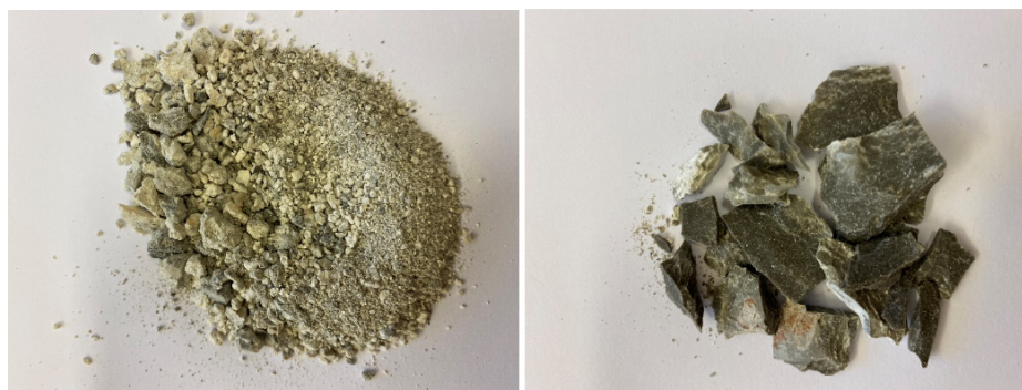
Figure 3.8: Grout gathered from different locations in the bridge [79].
