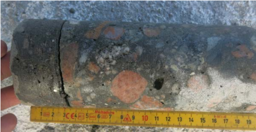
Figure 5-13 core A8 broken at the CP-mortar and bridge concrete interface
