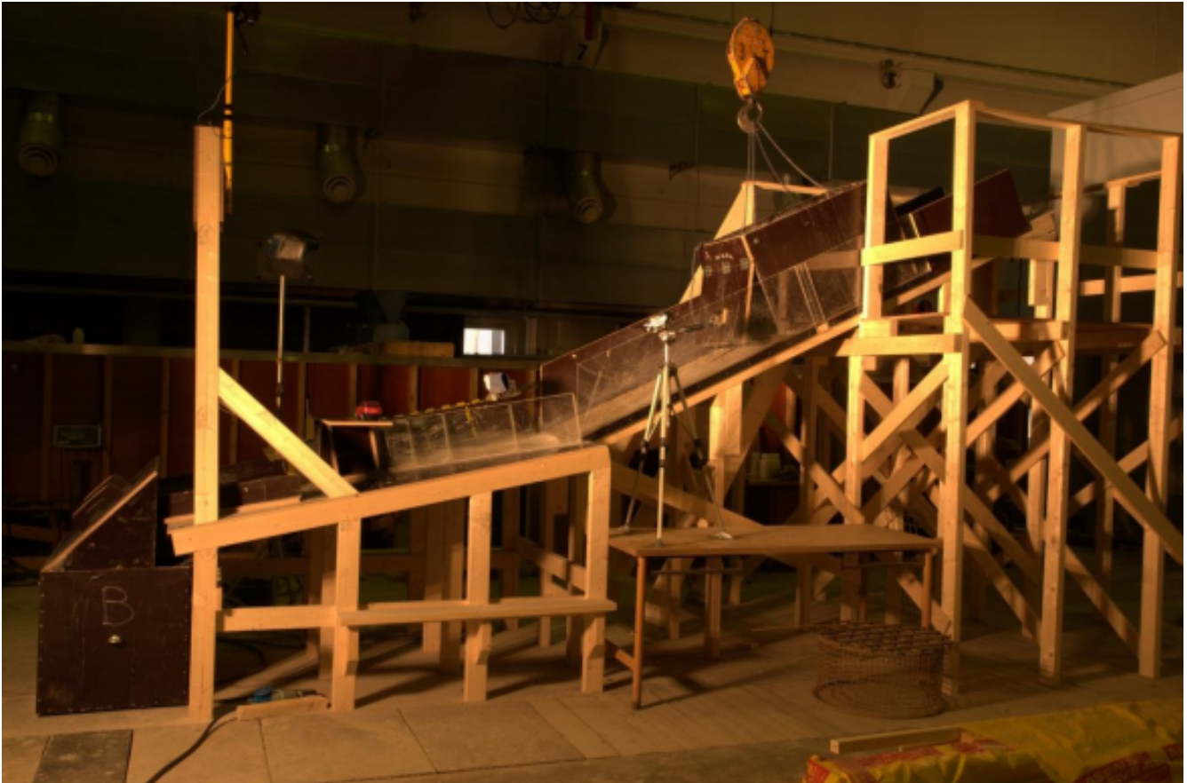
Figure 4.1: The debris flow model in 2009 when it was used to investigate the effect of channeling debris flows under a bridge by using deflection structures (Hiller and Jensen, 2009).
