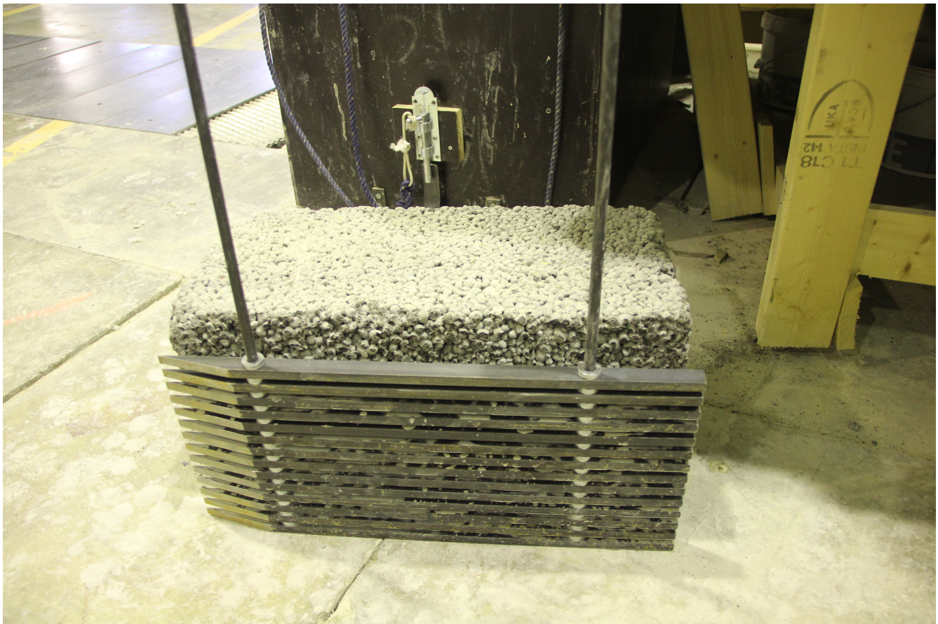
Figure 4.8: The 0.5 m long breaker leaning against a leca block while being built with 6 mm opening width.
