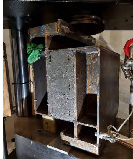
Wooden supports were used to safely position and stabilise the sample(s) until contact with the compression platens was achieved.
