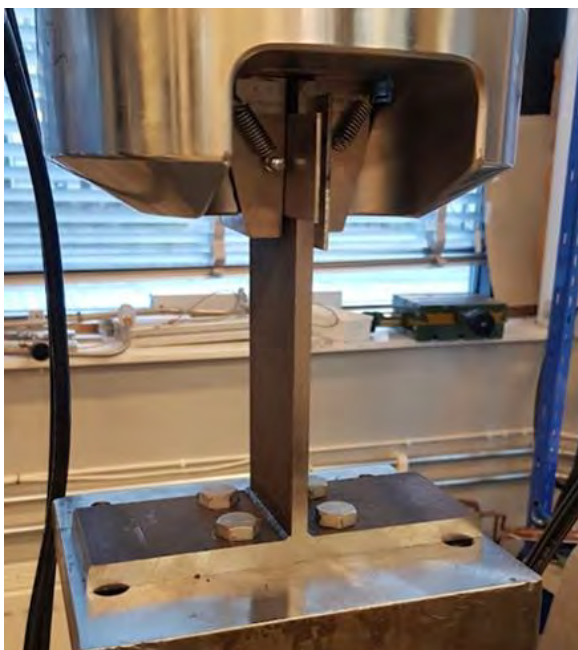
Figure 3. T-weld mounted in testing rig.
