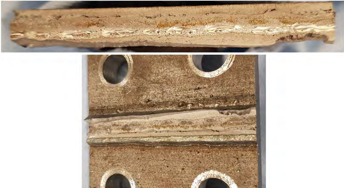
Figure 39. Fracture surface of T-weld 1 after fatigue testing.
