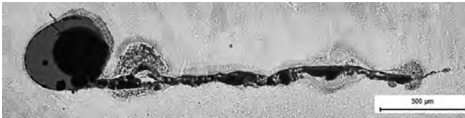
Figure 27. T-weld A from first delivery. Lack of fusion 2.5 mm, not permitted.
