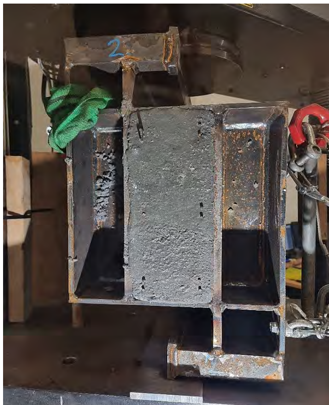
The sample after test. A visual of the shear failure in the casting. Thin line from the left upper corner to the right lower corner of the casting. Not so dramatic, which mirrors the graph on the previous page.
