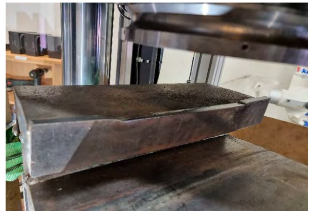
Deformation of the upper loading edge from the compression platen.
