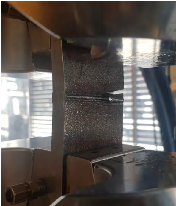
Figure 5. Fractured butt weld mounted in test rig.
