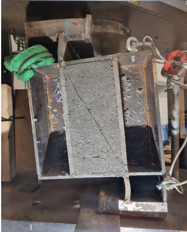
← The sample after test. A good visual of the shear failure in the casting.
