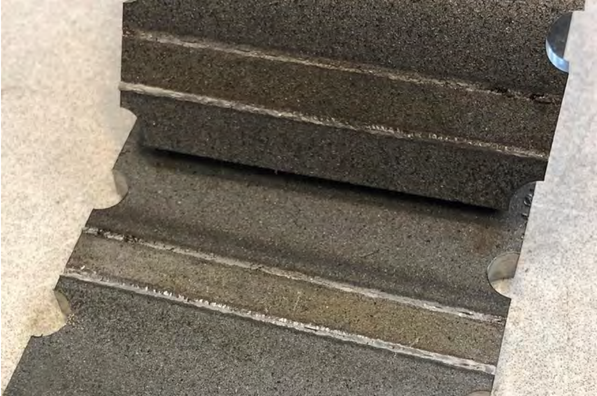
Figure 41. Fracture surface of stake weld after fatigue testing.
