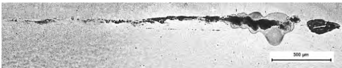
Figure 31. T-weld B from first delivery. Lack of fusion 2.8 mm, not permitted.
