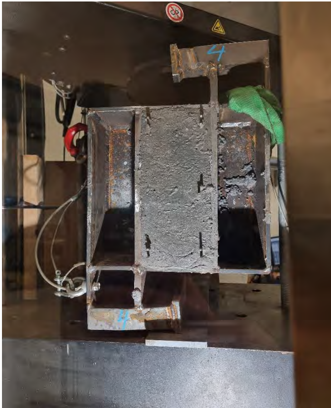
The sample after test. No visual on the outward facing surface of the shear failure.
