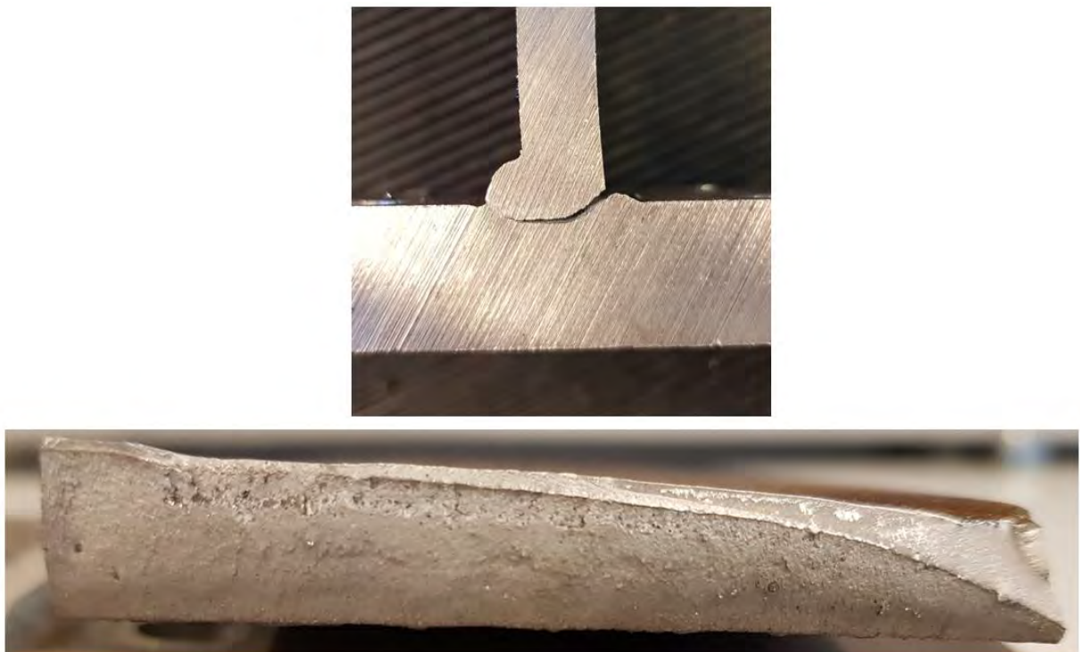
Figure 40. Upper: Crack propagation during fatigue testing of T-weld 2. Lower: Fracture surface after fatigue testing.
