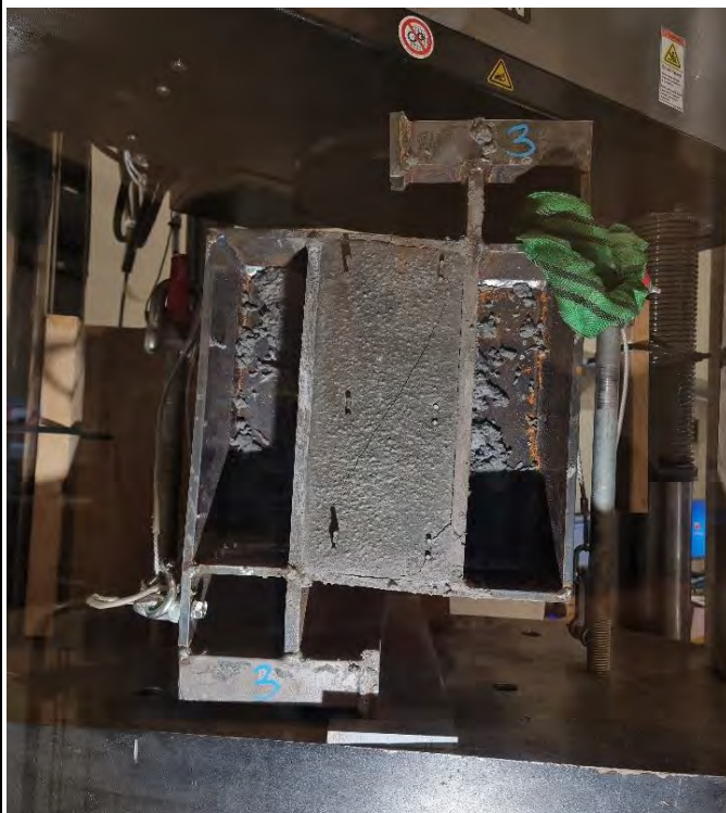
The sample after test. A good visual of the shear failure in the casting.
