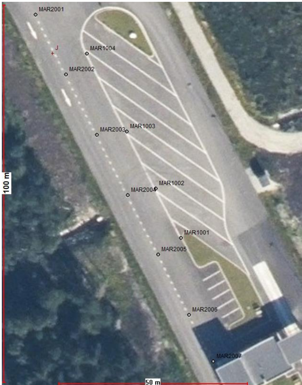
Figur 3 Overview of Marstein Controlstation with measurement points MAR2001 - MAR2007, verifying that the white dotted line is straight
