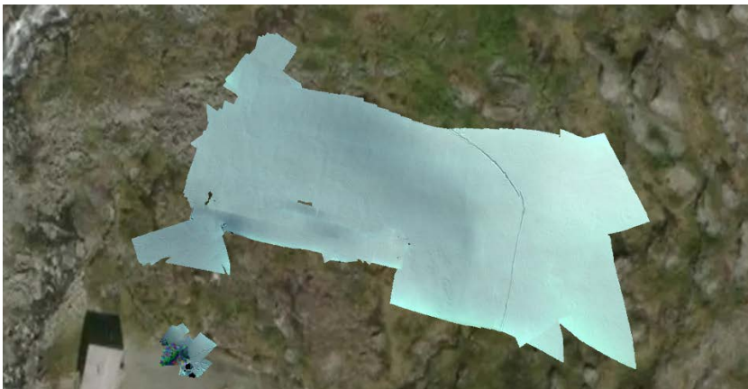
Figure 4-8. Colour images stitched together using Pix4D.
