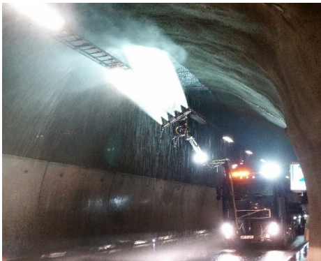
Figur 35: Vaskearm foran (Uniarm 700) (Foto: Terje Engstrøm)
