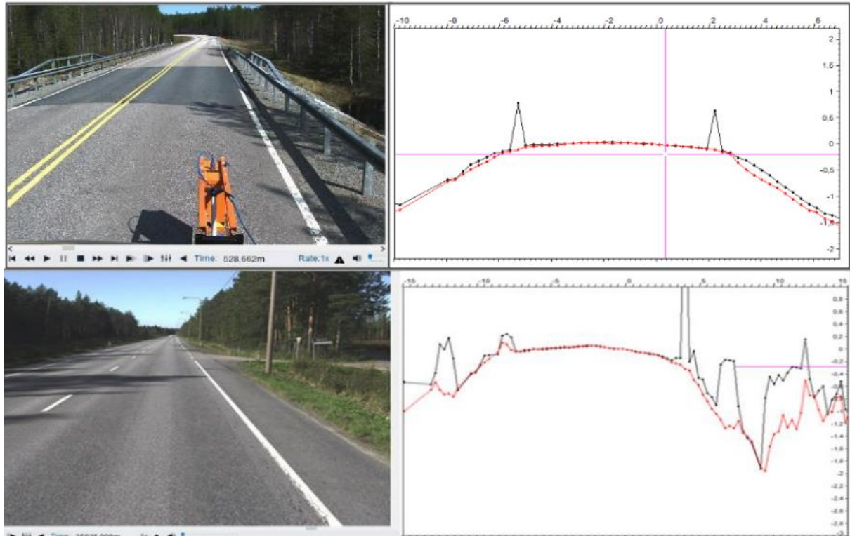
Figure 12. Cross sections from point clouds processed in two ways: Red line is drawn from the point cloud filtered so that rails and signs are removed, and effect of vegetation minimized. Black line is drawn from unfiltered point cloud showing all points.
