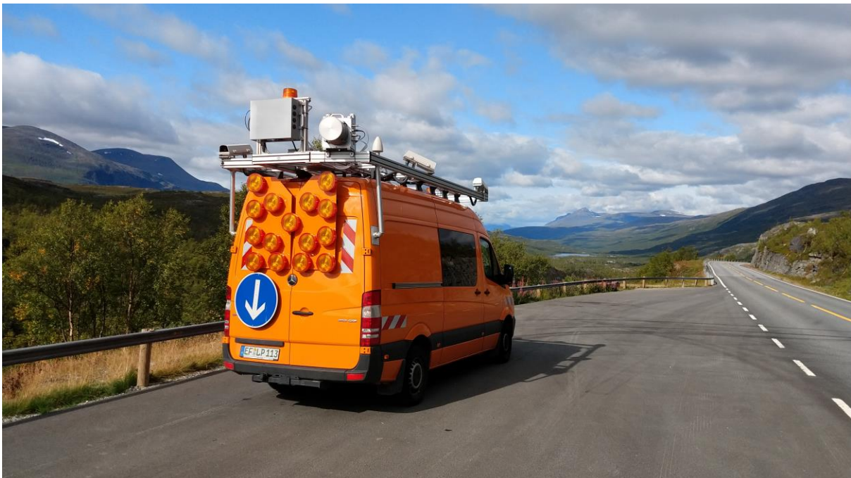
Figure 3: Mobile Mapping System I.R.I.S 13 with an inertial positioning system, several cameras and LiDAR sensors mounted on the roof rack. This image has been taken during the measurement on 22 nd August 2019 on E8.
