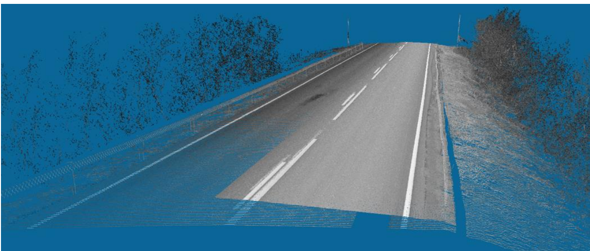
Figure 15:Perspective view along 3D point clouds from CPS (sparse points) and PPS+ (dense points).
