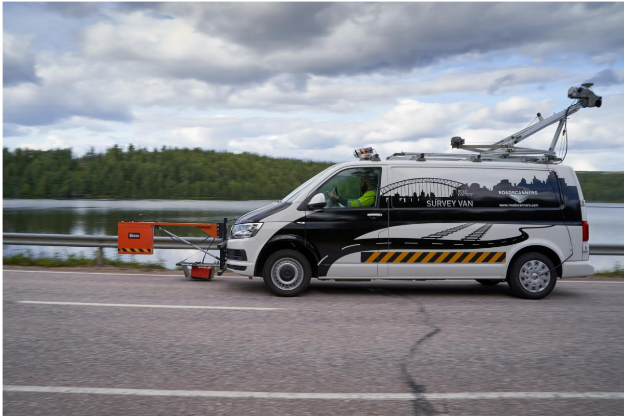
Figure 1. The Roadscanners GPR survey system equipped with a 2 GHz air coupled horn antenna and 400 MHz ground coupled antenna in the front of the vehicle. A video camera is mounted on the roof top and a laser scanner in the rear.
