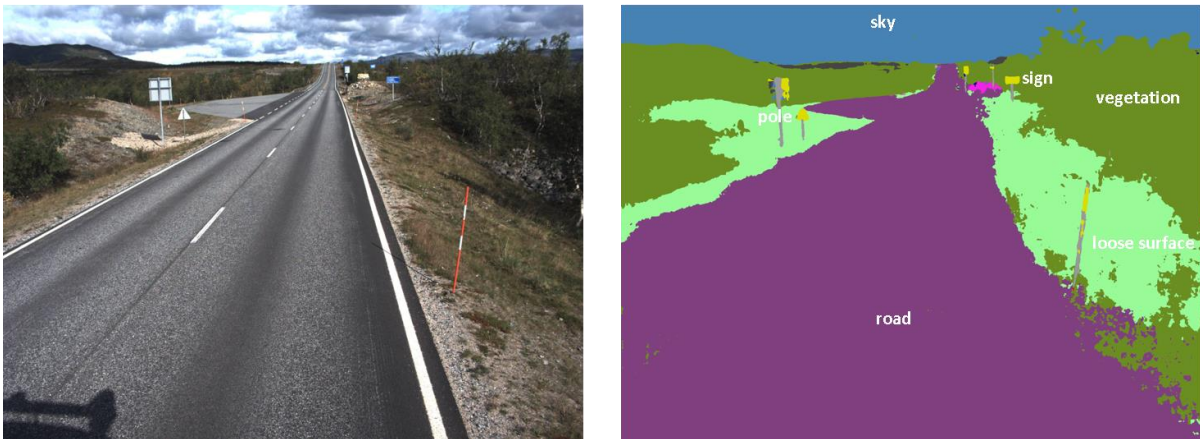
Figure 14:Automated object detection and classification on image data.
