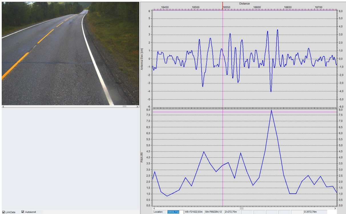
Figure 9. Screenshot from roughness data. Antenna elevation on top and accelerometer based IRI value at the bottom.
