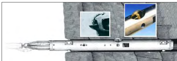
Figur 1.2.7-9: 2D-borehole slotter (Interfels)
