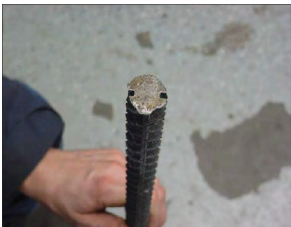
Figur 1.4.11-9: Maskinfreste slisser i kamstålbolt (B. Forbes)
