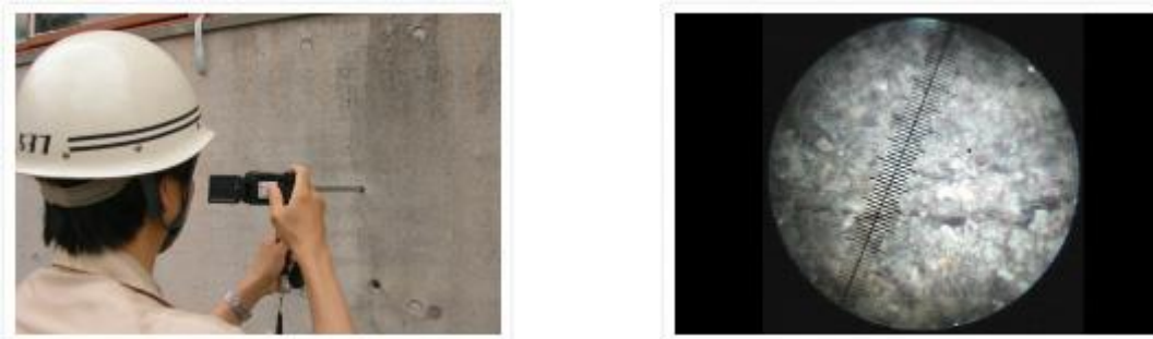
Figure 5.1 Use of endoscope, from ( http:// www.nishimatsu.co.jp )
