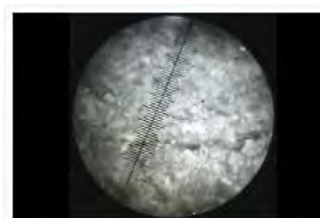
Figure 3.11 Use of endoscope identifying a crack in concrete, from ( http:// www.nishimatsu.co.jp )
