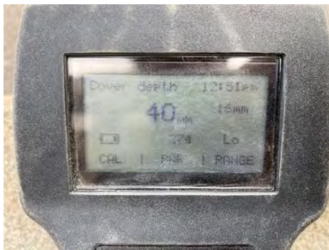
Figure 4.1 Cover depth determination with cover meter
