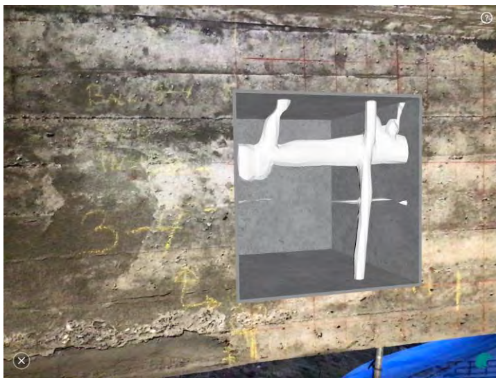
Figure 4.2: Example of 3D image of tendon duct with GPR
