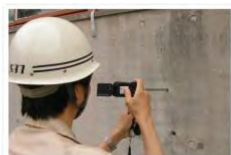
Figure 3.11 Use of endoscope identifying a crack in concrete, from ( http:// www.nishimatsu.co.jp )
