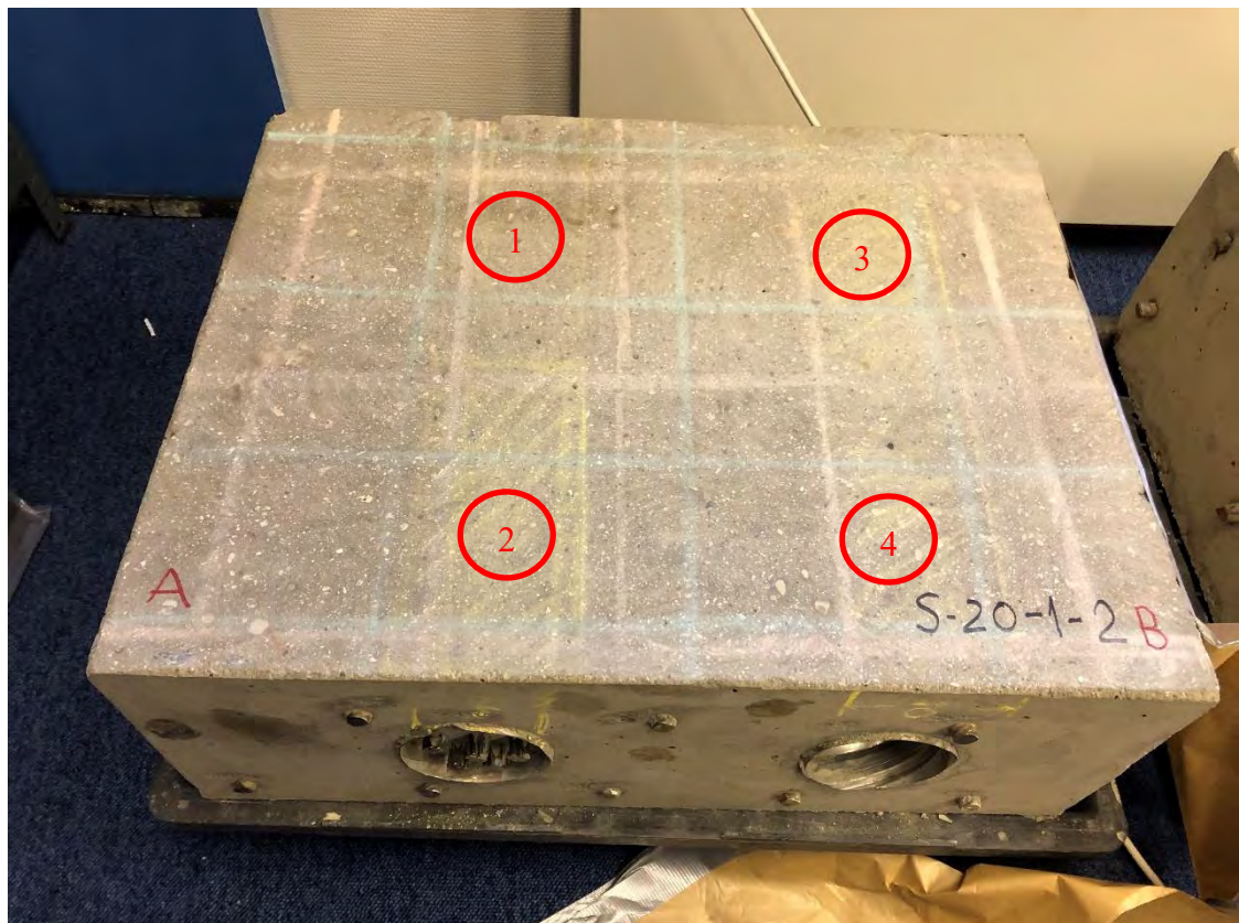
Picture 3.1: Placements of test points.
