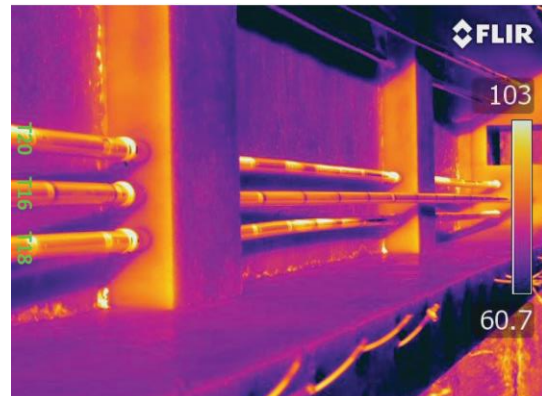
Figure 3.8 IRT Technique using FLIR T640 Infrared Camera and sample of infrared image of external tendons, from ( http://nap.edu/24779 )
