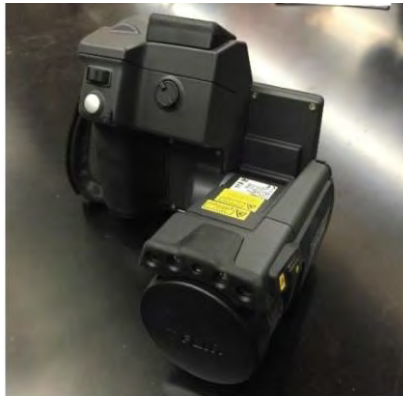
Figure 3.8 IRT Technique using FLIR T640 Infrared Camera and sample of infrared image of external tendons, from ( http://nap.edu/24779 )
