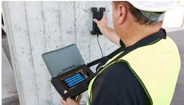
Figure 3.9 Use of cover meter, from ( http://www.proceq.com )
