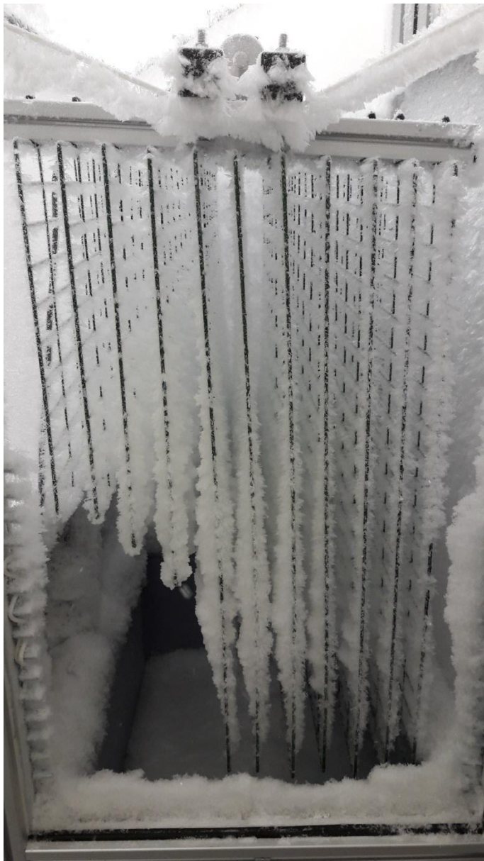
Figure 3: Plastic covered steel lattice inside of the Lumi where the snow gets created.
