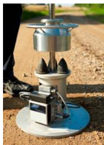
Figur 8.12 Portabelt fallodd (Foto: Impact test equipment)
