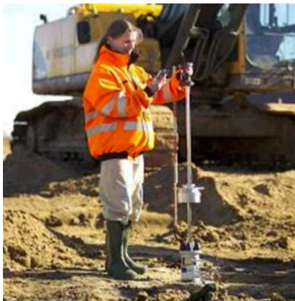
Figur 8.12 Portabelt fallodd (Foto: Impact test equipment)
