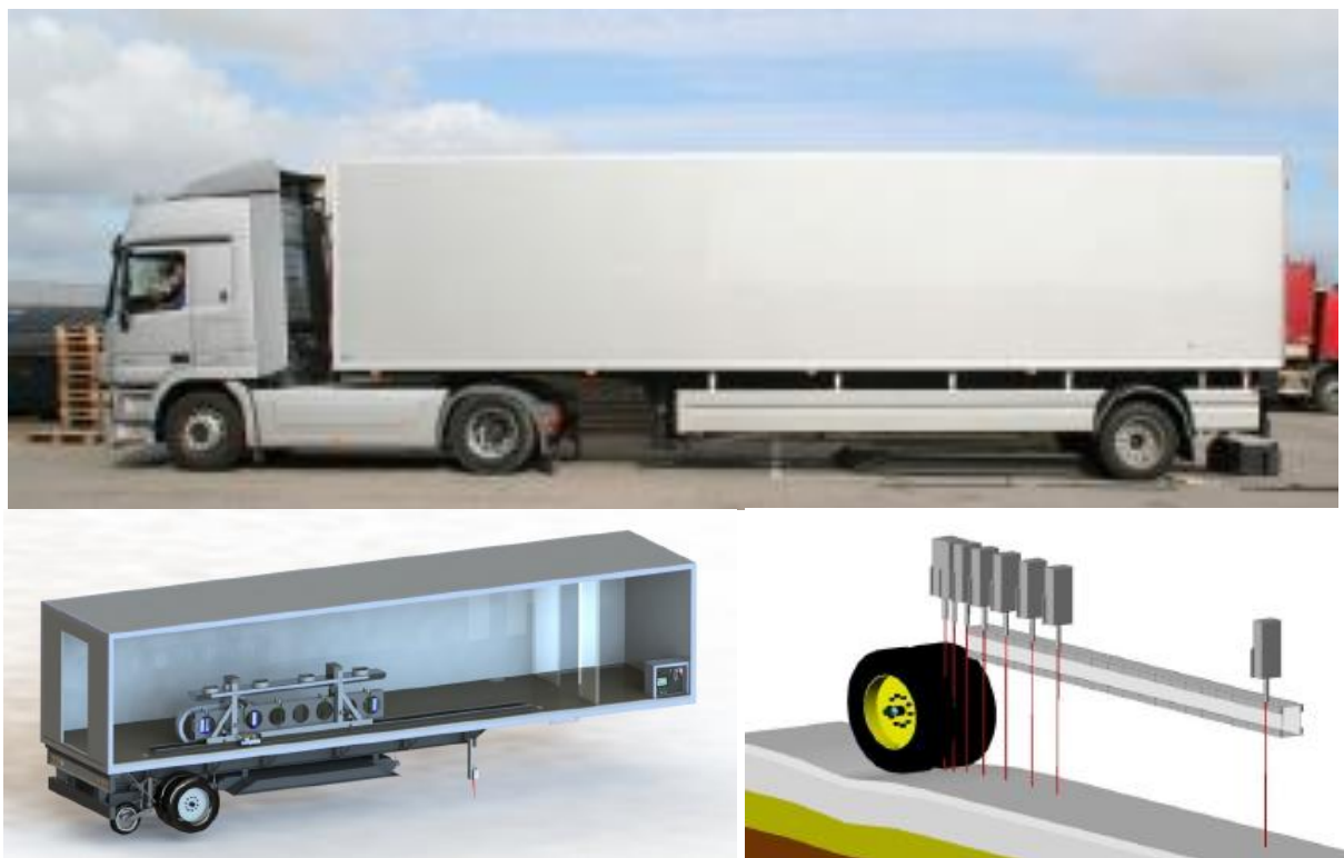
Figur 8.13 Traffic Speed Deflectometer – TSD (Foto: Greenwood.dk)
