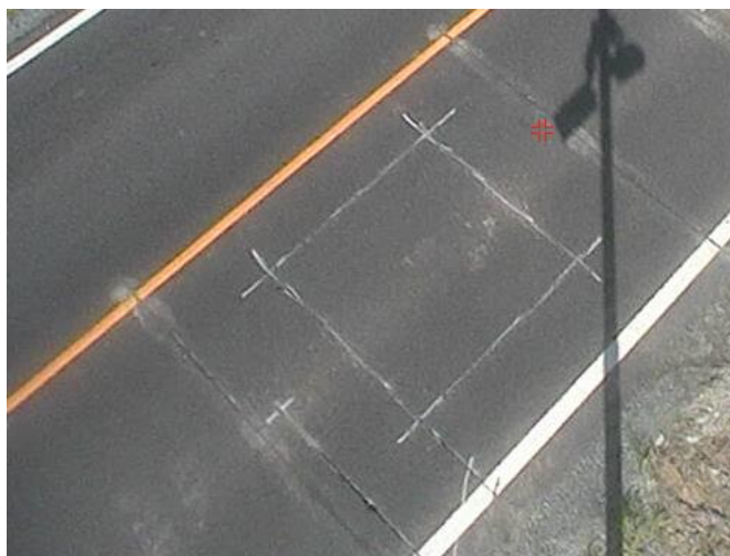
Figur 1 ViperWIM sensor layout, piezo-loop-piezo
