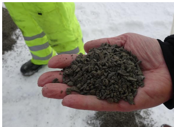
Figur 30: Dombås, knust fjell 2/6 mm.
