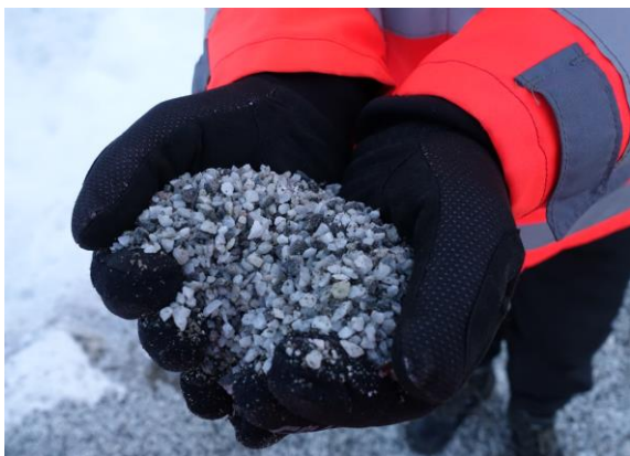
Figur 29: Visnes, knust strøsingel 2/7 mm.
